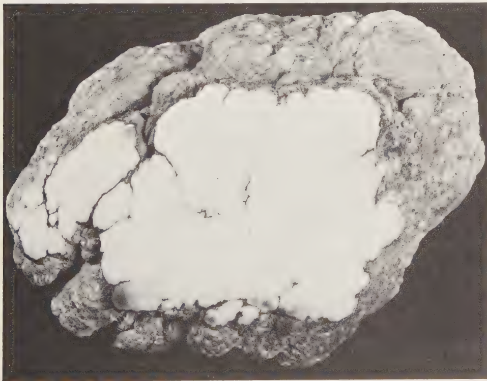
FIG. 197. Nodular mass of fine-grained howlite from the Sterling Borax Mine, Tick Canyon, Los Angeles County, California. Size 4" by 5". One portion of the nodule has been polished to expose the howlite.
