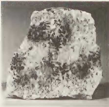
FIG. 158. Uraninite in pegmatite. The uraninite forms plumose and dendritic black growths surrounded by vividly-colored haloes of alteration products, mainly orange fourmarierite and vandendriesschite , and yellow becquerelite and schoepite . Sawed and lacquered section from the Ruggles Mine pegmatite, Grafton Center, Grafton County, New Hampshire. Size 3" by 3½".
