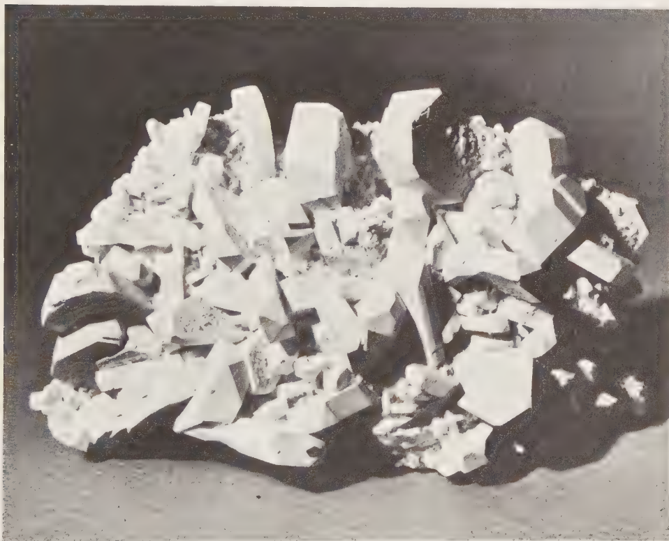
FIG. 193. Borax crystals on matrix of massive borax and clay from Boron, Kern County, California. Size 5" by 3". The white coating is tinalconite, to which mineral the originally transparent borax alters with exposure.
