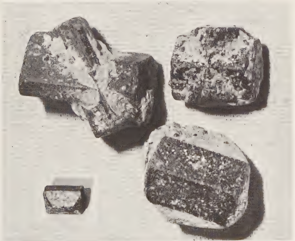
FIG. 315. Staurolite crystals from Pilar, New Mexico, showing two modes of twinning. Crystals are obtained from within mica schist, some of which still adheres to specimens. Largest crystal about 1" diameter. The inset photo shows a small single crystal from Fannin County, Georgia. Photo courtesy Scott Williams Mineral Company, Scottsdale, Arizona.
