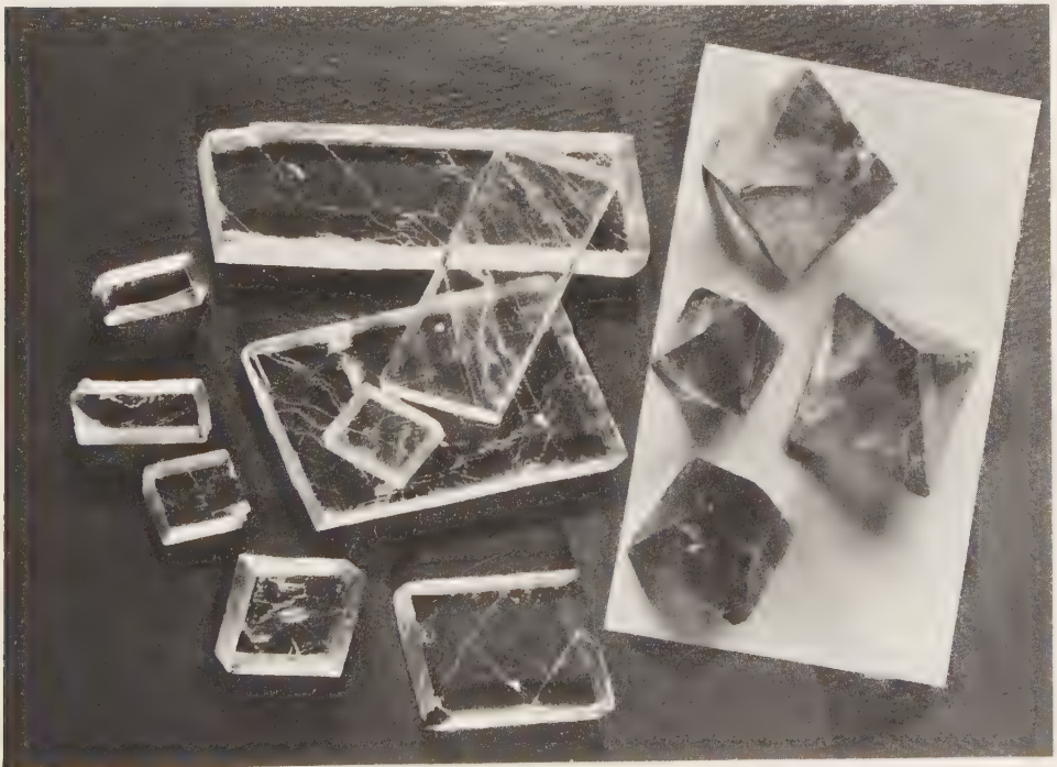
FIG. 78. Cleavages in Fluorite and Calcite. The inset shows nearly perfect octahedrons obtained by carefully cleaving larger cubic fluorite crystals. Below are cleavage rhombs of colorless calcite, several of which show doubling of images due to the strong double refraction of this mineral. Inset photo courtesy Schortmann's Minerals, Easthampton, Massachusetts.
