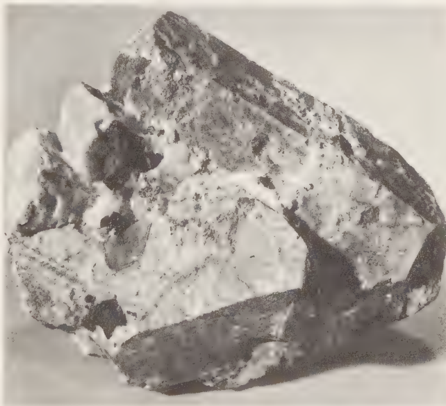
FIG. 307. Hexagonal prisms of brown willemite, variety troostite , in calcite, garnet and franklinite matrix, from Franklin, Sussex County, New Jersey. Size 6" by 5".
