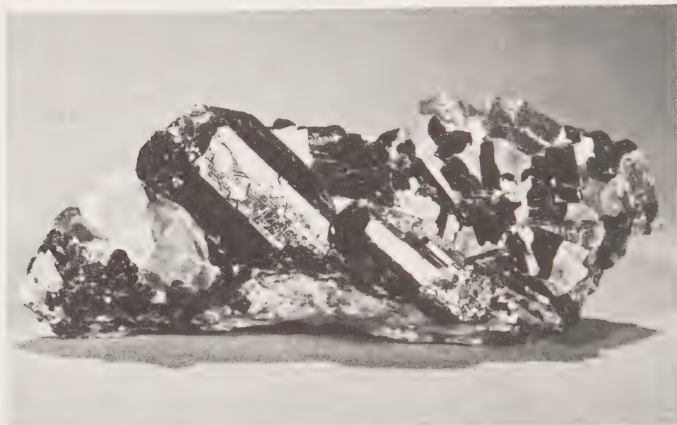
FIG. 278. Dark green diopside crystals in calcite with chalcopyrite, apatite and fluorite. Size 3\frac{1}{4} " by 1\frac{1}{2} ". From Huddersfield, Quebec. Crystals are rounded on edges, as if partly fused. Elongated along the c axes. Prism zone bounded by prism m[110] and pinacoids a[100] and b[010] .
