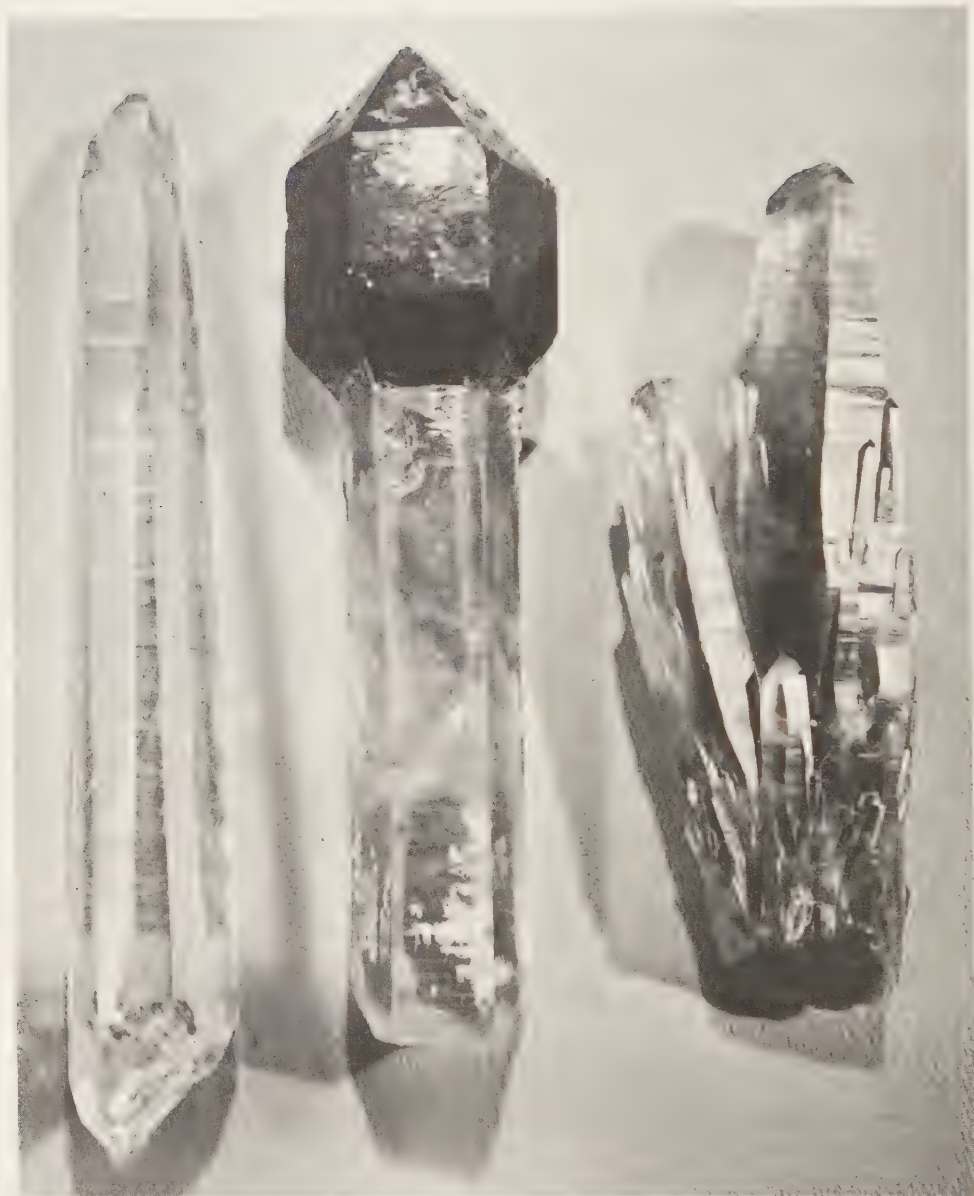
FIG. 239. Quartz crystals. Left : doubly-terminated rock crystal "candle," showing hexagonal cross-section at the bottom, gradually tapering and obliterating one set of m[10\bar{1}0] faces until the cross-section at the top is triangular. From Minas Gerais, Brazil. Length 9\frac{1}{4} ". Center : magnificent scepter quartz displaying smoky quartz overgrown upon slightly smoky stem. From Minas Gerais, Brazil. Length 9". Specimen from the Alice J. Walters Collection, Ramona, California. Right : tapering amethyst crystals from Santa Margarita Mine, Guerrero, Mexico. Length 7".
