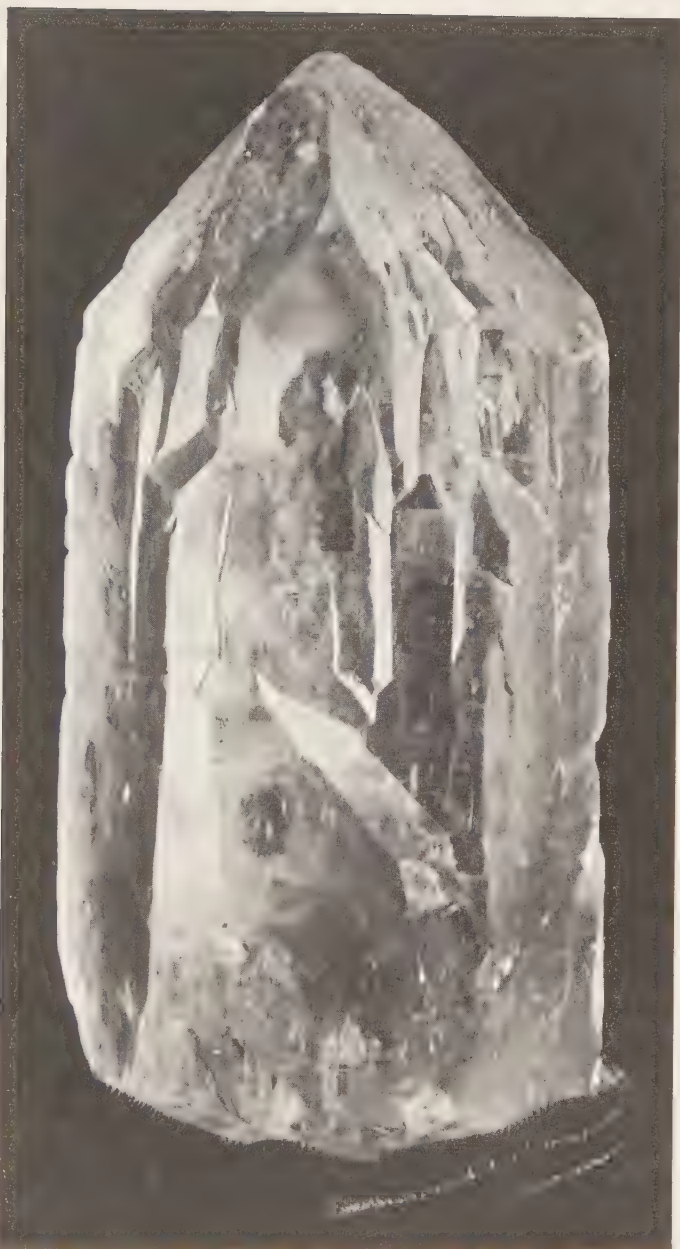
FIG. 44. Dauphiné twinning in quartz. A 7" rock crystal from the San Pedro Mine, Hiriart Hill, Pala, San Diego County, California, showing the many steps and offsets produced along the sides and top as the result of numerous dauphiné twins.
