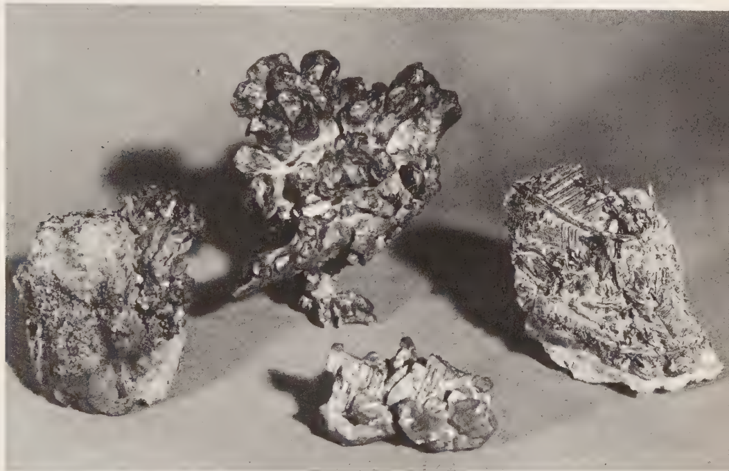
FIG. 109. Native silver and copper. Left : crystals of copper on limonite matrix from Campbell Shaft, Bisbee, Cochise County, Arizona. Size about 2" by 1½". Bottom center : native copper crystals showing hopper development. Size 1¾" diameter. New Cornelia Pit, Ajo, Pima County, Arizona. Top center : native silver in rude branching crystals from Wolverine Mine, Cheboygan County, Michigan. About 3" by 2¾". Right : arborescent silver forming sprays of twinned crystals in limonite matrix on limestone. About 2¼" by 2". Batopilas, Chihuahua, Mexico.
