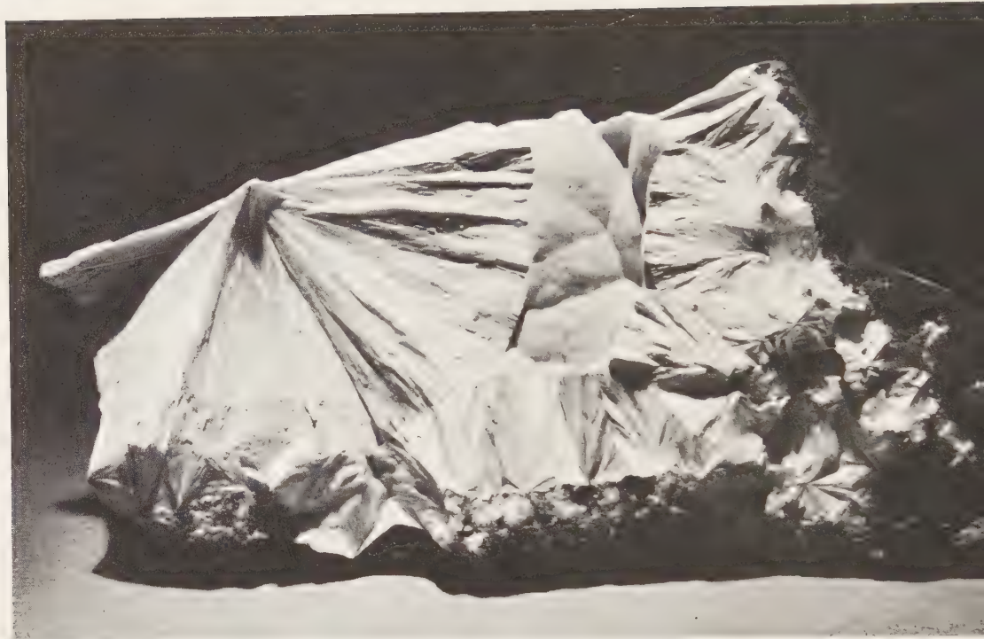
FIG. 282. Pectolite on basalt from Prospect Park, Paterson, Passaic County, New Jersey. The radiating structure is well shown here, while in the center of the specimen appear the spherical surfaces which face inward from cavity walls. Size 5" by 3".
