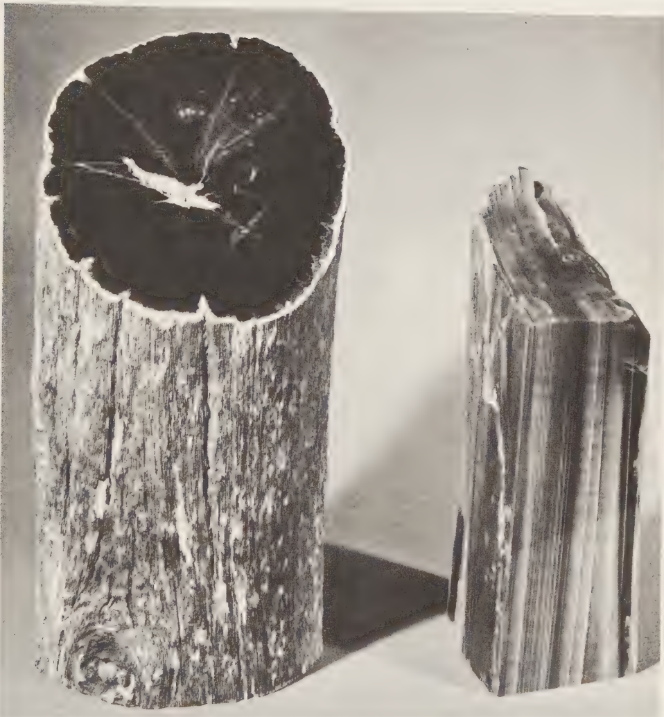
FIG. 244. Wood replaced by chalcedony. Left : oak from Eden Valley, Sweetwater County, Wyoming. Size 6¼" tall, 3" diameter. Right : silicified cypress from the state of Washington. Size 5" by 1¼" by 2½". Both specimens display very faithful replacement by quartz, the cellular structure being perfectly distinct.
