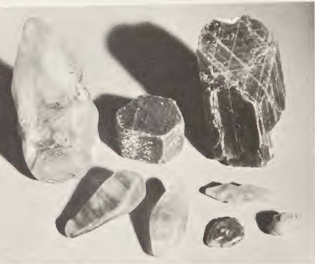
FIG. 146. Corundum crystals. Top and bottom left : large water-worn crystals from the gem gravels of Ceylon; the larger dipyramidal crystal at upper left is yellow in hue and measures about 3" tall. Top center : tabular hexagonal prism of ruby corundum from Matabatu Mountains, Tanganyika. Top right : dark blue parting fragment from Mozambique showing parting parallel to c(0001) at the top of the specimen, and partings on the sides parallel to the rhombohedron r(10\bar{1}0) . Lower right : an irregular dipyramidal crystal from Ceylon and two ruby crystals from Mogok, Burma.
