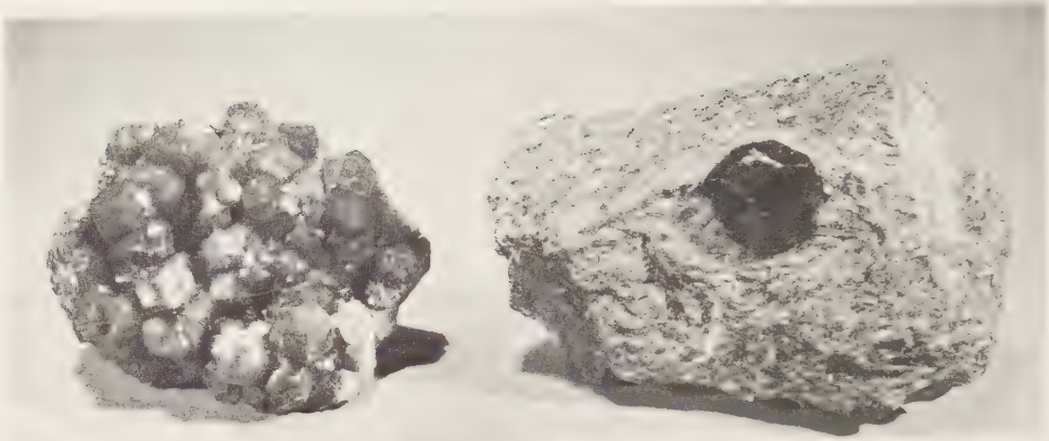
FIG. 317. Garnet specimens. Left : dodecahedral crystals of brownish andradite from Stanley Butte area, Graham County, Arizona. Size 2" by 2". Right : dark red crystal in mica schist from near Wrangell, Alaska. Forms are the dodecahedron modified by the trapezohedron. Size 3½" by 2½".
