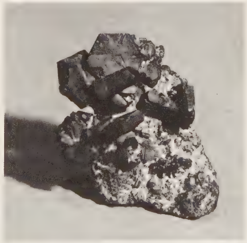
Fig. 114. Chalcocite sixling twins on matrix of massive chalcocite, from Messina, North Transvaal, South Africa. Size of specimen 1\frac{1}{2} ". Note striations on the c(001) plane of the crystal at the top.
