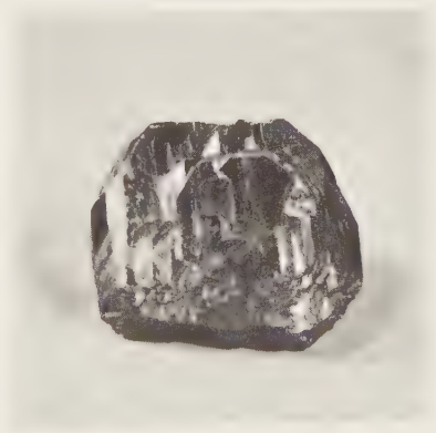
FIG. 171. Columbite. Several lustrous black crystals growing in sub-parallel position. The broad faces are b(010) . Minas Gerais, Brazil. Size 1\frac{1}{2} " by 1".
