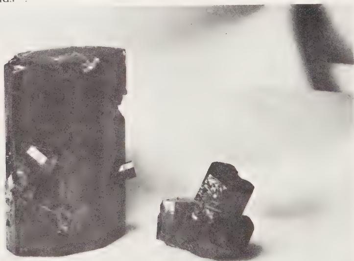
Figure 9.3 Gilson emerald single crystal and cluster after ten months' growth. The large crystal measures about 63 mm (2½ in) tall and 37 × 12.5 mm (1½ × ½ in) in cross-section; several spontaneously seeded crystals are attached. The cluster crystals show development of second order prisms. Courtesy Laboratoire Gilson.
