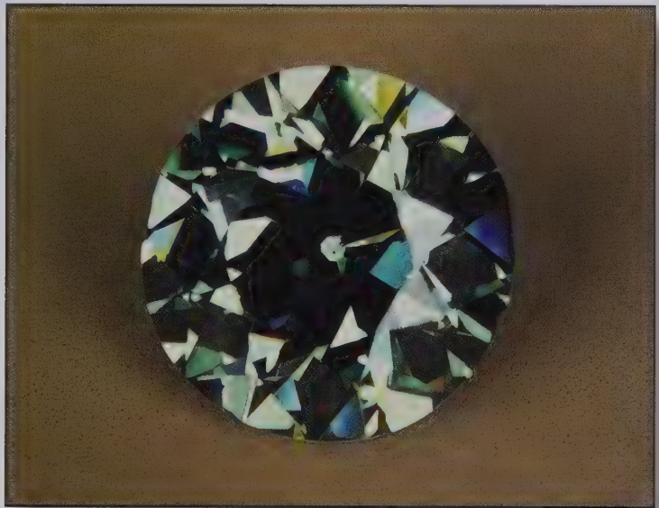
Diamond exhibiting darkness beneath the table, known as the fisheye effect. Note the bright spot at the center of the table, that is a window caused by a flat faceted culet.
