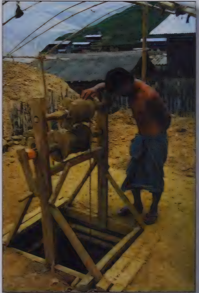
Traditional mining in the ancient 'Valley of the Serpents' Mogoke, Burma. This age-old mining method consists of a wooden, hand-dug vertical shaft drops forty feet to the gem-bearing layer, or floor, where a narrow horizontal shaft is dug into the gem gravel. The gravel is raised by buckets and sorted. Photo: B. W. Mac
