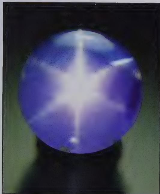
A 14.40 carat blue star sapphire exhibiting a very well formed six-rayed star. The hexagonal arrangement of rutile inclusions responsible for the phenomenon is visible in the background. Photo: Jeff Scovil, courtesy Mine Design.
