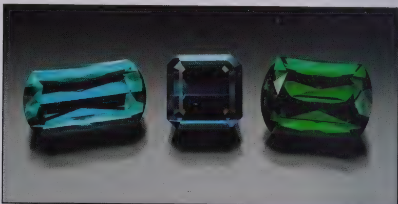
Three green tourmalines photographed in incandescent light. The two stones at either end maintain their transparency, the center stone closes up and turns sooty. Note the elongated bow-tie shaped black bands of extinction in the stones to the left and right. Photo: Jeff Scovil, courtesy R. W. Wise, Goldsmiths.
