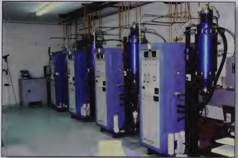
High tech ovens used in the heat treatment of Montana sapphire. Except for precision control of temperature and duration, the technique differs little from that described by Al Beruni. Photo: R. W. Wise.
