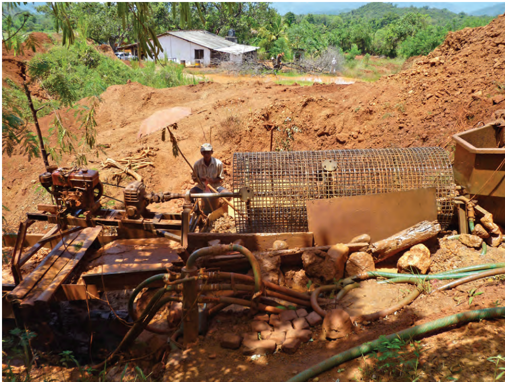
Mechanised mining is no longer allowed in Sri Lanka, but some licence holders have permits that predate the current law. Using an apparatus consisting of a washing basin, trommel, and jigs, the gems are collected in pans beneath the jigs. A scene from the Elahera gem fields. (Photo: Cynthia Unninayar)
