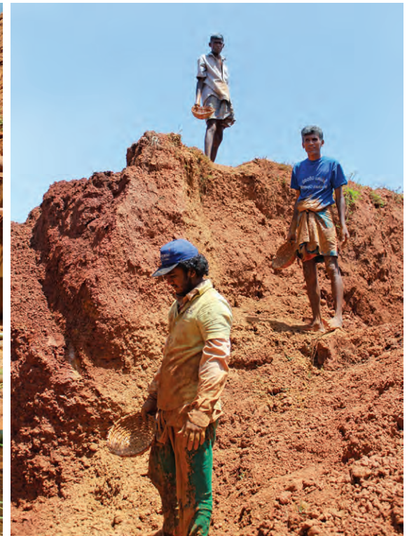
In artisanal mining, the miners transfer the gem material in baskets from one person to another from the bottom of the wide pit to the top at the Elahera gem fields. (Photo: Erica Courtney)
