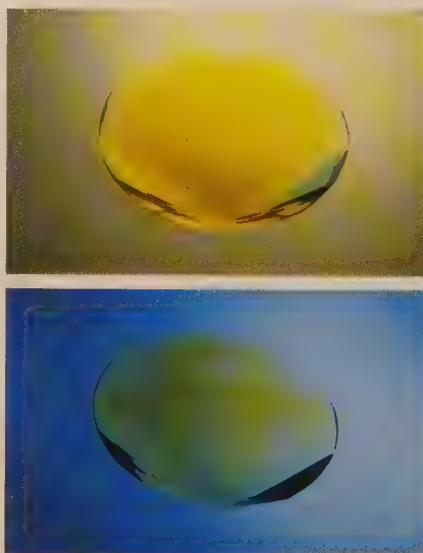
**Figure 7.38** Inserting a frosted blue filter beneath the immersion cell makes locating color zoning far easier in yellow stones. **Top:** With normal lighting, the yellowish light combined with the yellowish color of the immersion liquid combine to obscure color zoning. **Bottom:** Imposition of a blue filter quickly reveals the curved color banding of this Verneuil synthetic yellow sapphire. (Photos by the author)
