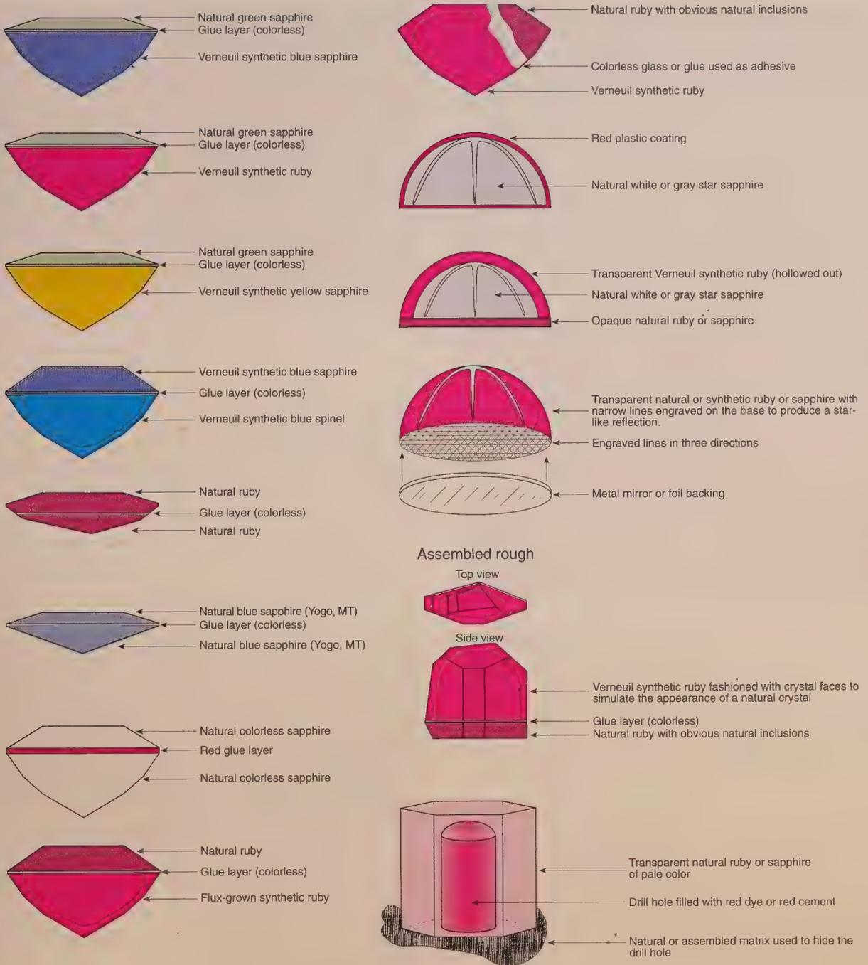
**Figure 8.3** Commonly-encountered examples of assembled rubies and sapphires. Other combinations are also possible, but these represent the types most frequently seen.
