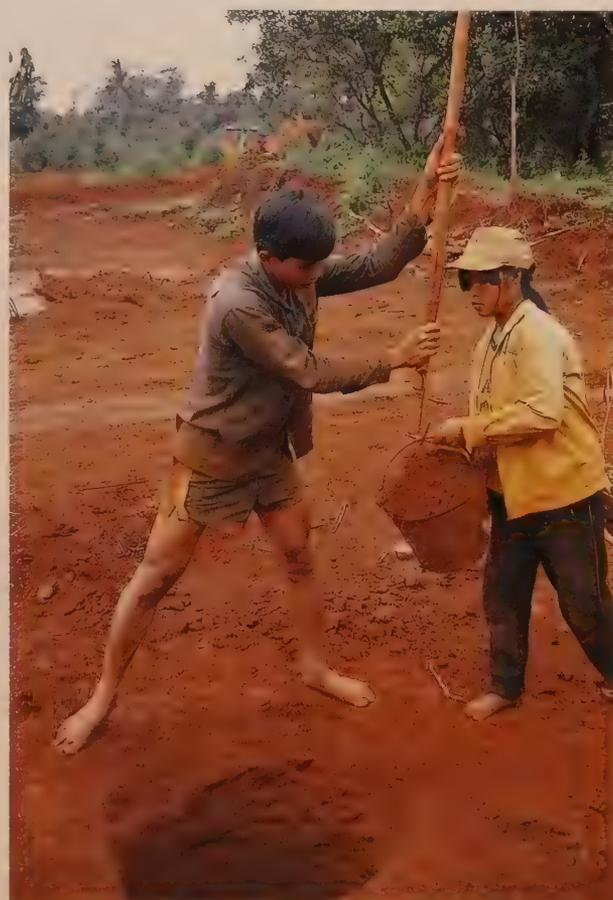
Figure 12.121 The traditional method of mining is to sink a pit down to the gem-bearing layer. All that is needed is a partner, a few simple tools and, most importantly, the dream of finding sapphires. Here, miners work in the shadow of Khao Ploi Waen, the "Hill of Gems." (Photo by the author)
