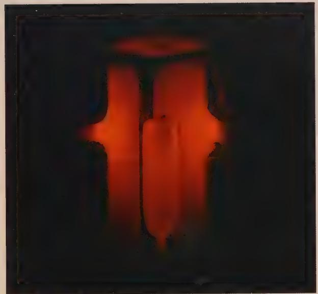
**Figure 7.4** Verneuil boule in the furnace just after the torch has been turned off. (Photo: Djehahirdjian)
