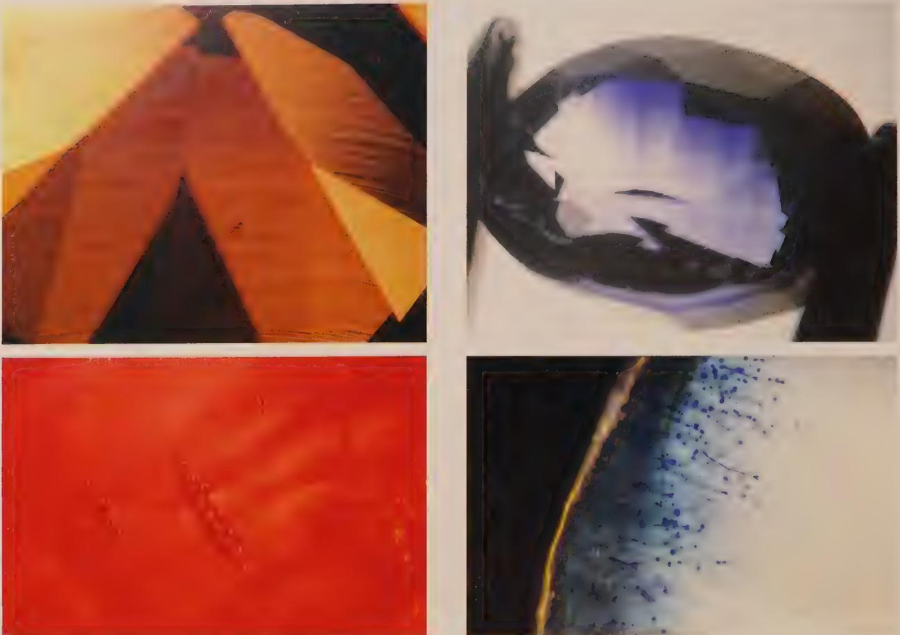
**Figure 7.11** The key that unlocks the Verneuil product's identity—curved growth lines and gas bubbles
