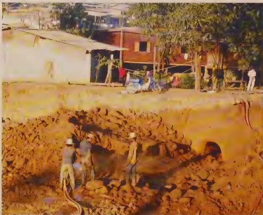
**Figure 12.130** Ruby mining in Thailand proceeds at a frantic pace, sometimes even beneath miners' huts. Here, miners at Nong Bon (Trat Province) use a water cannon to pump the ruby-bearing soil into a tunnel running right beneath their homes. On the other side, a jig will separate the rubies and heavier minerals from the worthless overburden. (Photo by the author, ca. 1983)
