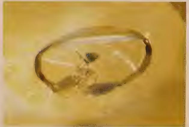
**Figure 5.4** Two views of a primary negative crystal in a Sri Lankan sapphire. The cavity contains liquid and gaseous CO<sub>2</sub>, along with a mobile graphite crystal cluster. In the top photo, a CO<sub>2</sub> bubble is clearly visible, while in the lower photo the CO<sub>2</sub> bubble has disappeared from the gentle heat of the microscope. The black graphite crystals can also be seen to have moved in the lower photo. (Photos: John Koivula/GIA; 35X)
