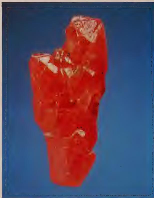
**Figure 2.13** 4.75 cm long ruby crystal from Luc Yen, Vietnam. Note the rhombohedral twinning striations, which are common on many corundum crystals. (Photo: Tino Hamid/GIA)
