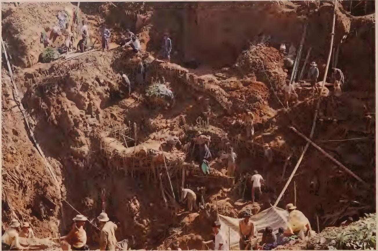
**Figure 11.11** Despite the wonders of modern technology, much gem mining is still performed by simple techniques, such as those used on this hillside mine at Inn Gaung, in Burma's Mogok Stone Tract. (Photo: Thomas Frieden)
