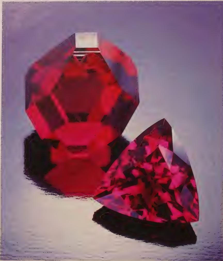
**Figure 7.22** Masterpieces of the crystal growers' art. The 8.77-ct crystal at the rear is a rare example of a near-perfect rhombohedron. In the foreground is a 3.67-ct faceted stone. Both are Ramaura flux-grown synthetic rubies. Unlike melt synthetics, the slow growth of solution processes produces stones which more closely resemble those of nature. (Photo: © 1983 Tino Hammid/GIA)
