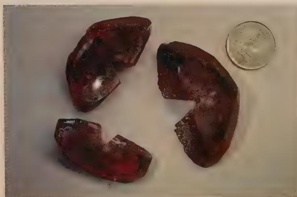
**Figure 7.29** Rough flux-grown Kashan rubies. Note the V-shaped cuts at the center of each where the seed crystal was originally located. (Photo: Tony Laughter)
