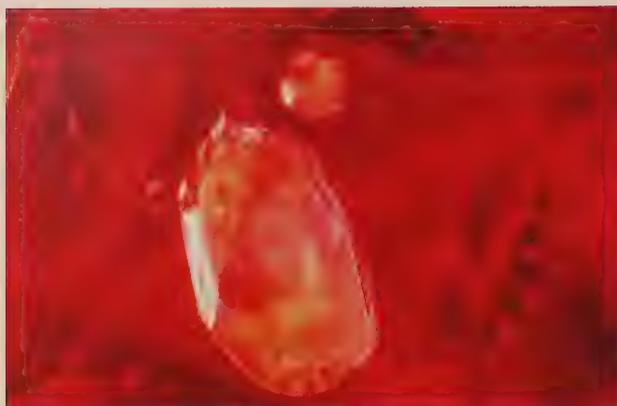
**Figure 12.49** A large crystal of calcite in an unheated Mogok ruby, in polarized light. Calcite is suggested because of the intersecting twinning planes visible within the included crystal. Such calcite crystals containing repeated glide twinning are often seen in Burmese rubies, which were formed in a calcite (marble) matrix. (Photo by the author)
