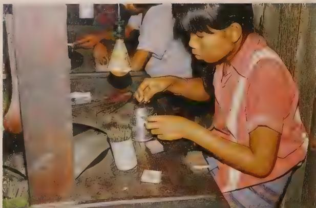
**Figure 9.5** The faceting method widely used in Thailand today was introduced to the country by a Dutch diamond cutter named Zerner shortly after World War II. Thus the equipment bears a strong resemblance to that used by diamond cutters. The Thai cutter above is dopping the stone prior to faceting. (Photo by the author)
