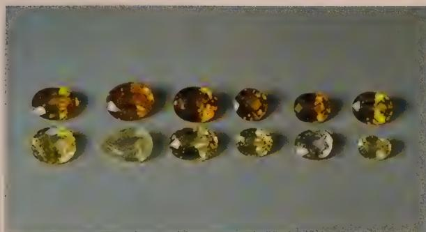
**Figure 6.24** Fading behavior of irradiated Sri Lankan yellow sapphires. Stones in the top row are pictured before fading and those in the lower row have been subjected to a fade test. (Photo: Tony Laughter)
