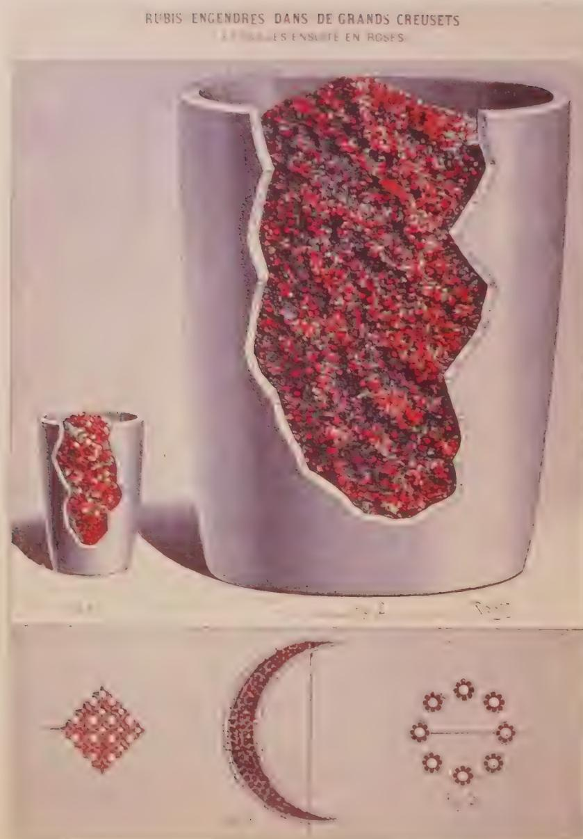
**Figure 7.1** Plate from Edmond Fremy's book on the synthesis of ruby. It shows a crucible filled with tiny flux-grown rubies. Below is jewelry incorporating small examples of these rubies. (Photo: Robert Weldon/GIA)
