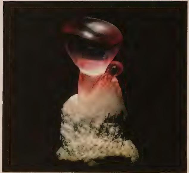
**Figure 7.7** Verneuil synthetic ruby boule still sitting on the sinter cone. (Photo: Mike Havstad/GIA)
