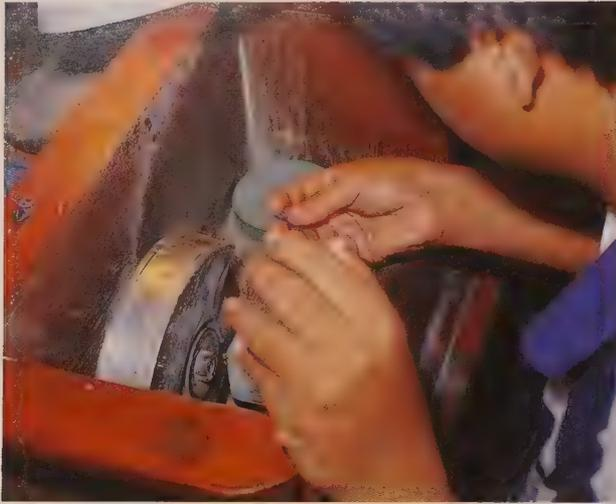
**Figure 9.1** Preforming is the most important step in cutting because it is here that the gem is given its essential shape. Pictured is a Thai lapidary preforming blue sapphire on a grinding wheel. (Photo by the author)
