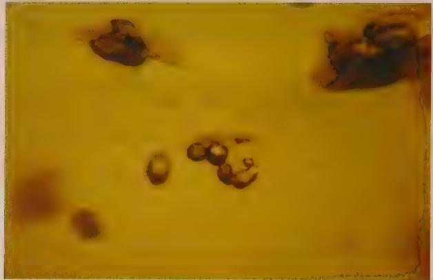
**Figure 12.98** Zircon is one of the most common solid inclusions found in Sri Lankan corundums. These tiny crystals often display tension haloes, which are believed to result from expansion of the zircon due to metamict (radioactive breakdown) processes. (Photos by the author)
