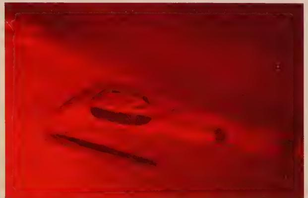
**Figure 6.12** During heat treatment, solid inclusions will melt if their melting point is below the maximum temperature reached. Due to the rapid cooling rate of the oven, these inclusions generally cool into a glass. Because the glass takes up less volume than the previous crystal guest, gas bubbles form to fill the remaining space. In the heated Thai/Cambodian ruby above, several gas bubbles can be seen in this melted crystal inclusion. (Photo: Wimon Manorotkul)
