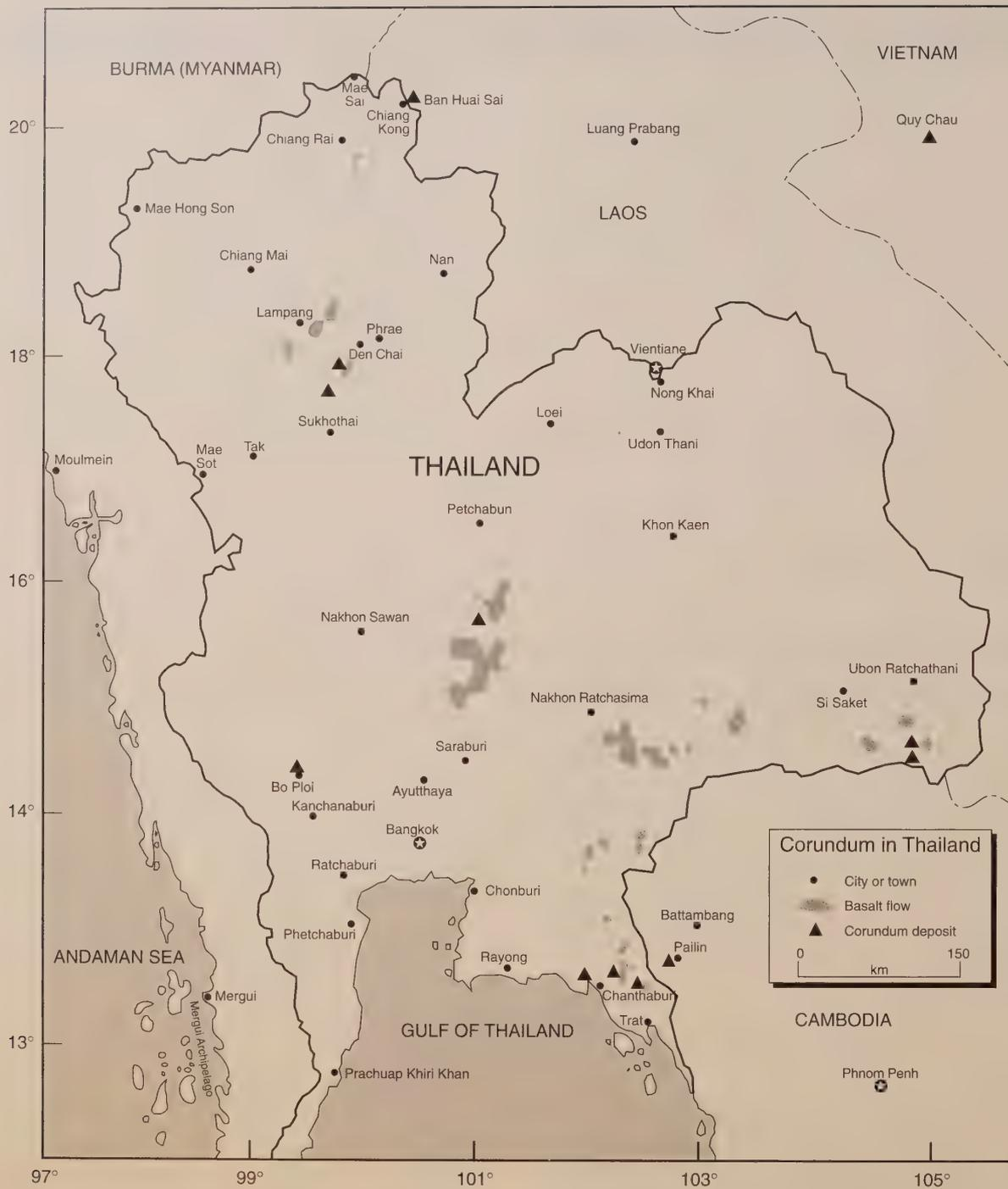
Figure 12.113 The corundum-producing localities of Thailand, eastern Cambodia and Laos. (Modified from Vichit & Vudhichativanich *et al.*, 1978)
