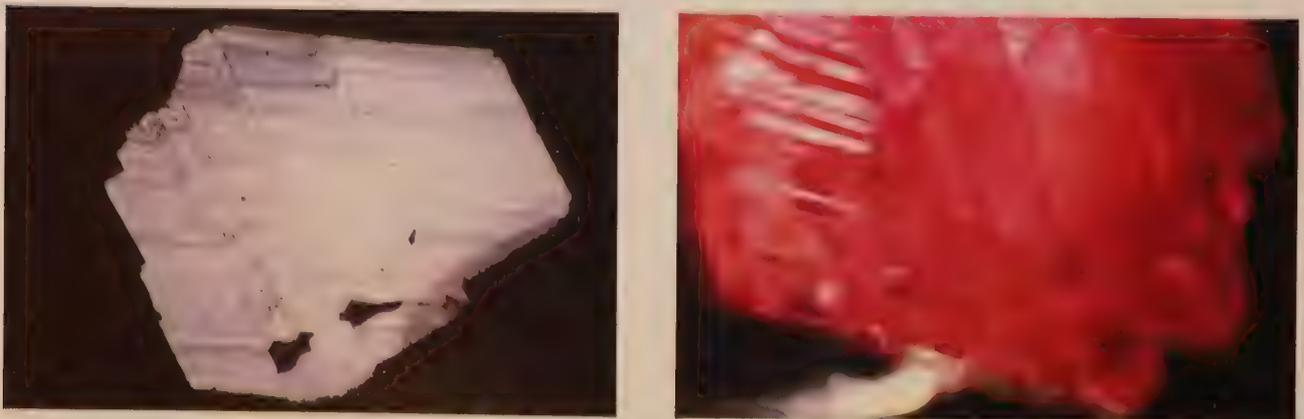
Figure 7.33 Lechleitner synthetic flux corundum overgrowth on a natural seed
