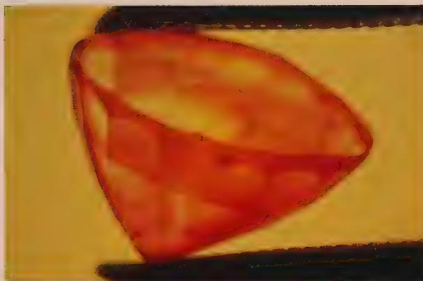
**Figure 6.19** Red SDTC immersed in di-iodomethane. Note the obvious patchy color concentrated on the surface. (Photo: Tony Laughter)
