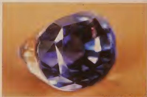
**Figure 8.2** Doublet? Not hardly. This stone is an *ottu* blue sapphire from Sri Lanka. The color is concentrated near the cutlet, but because of reflections, it appears that all the color is in the crown. To properly identify an assembled stone, one must locate the separation plane, rather than just a difference in color. (Photo: GIA)
