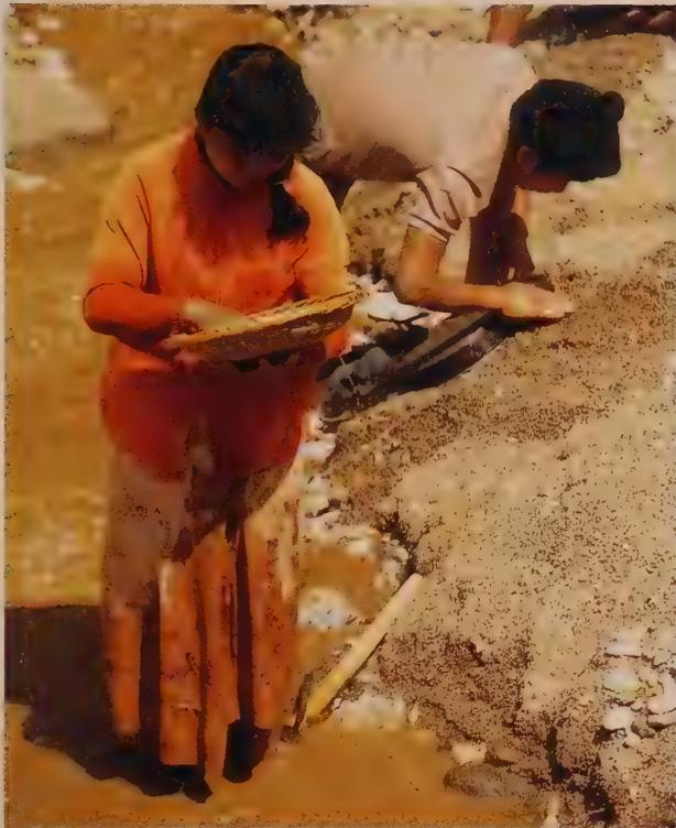
**Figure 12.38** Washing gem gravels in a stream in Burma's Mogok Stone Tract. (Photo: Robert Kammerling/GIA)
