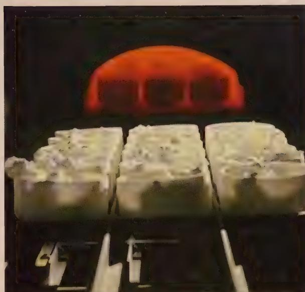
**Figure 7.6** Alumina powder heading into the drying furnaces prior to the production of Verneuil synthetic corundum.
