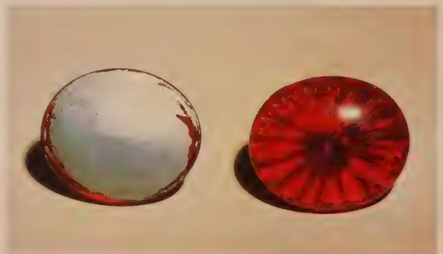
**Figure 8.5** Synthetic ruby foilbacks. This type actually consists of a special foil paint applied to increase brilliance. (Photo: Tino Hammid/GIA)
