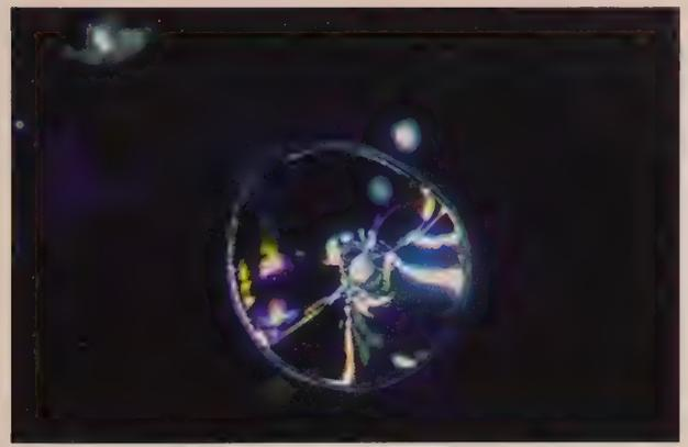
**Figure 6.11** Tension disks in heat-treated corundums
