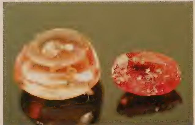
**Figure 6.8** Evidence of the high temperatures reached during modern heat treatments is found in the above photo of heated Sri Lankan rubies. One can clearly see the melted surfaces, solidified droplets and fragments of stone that have been fused to the surfaces of these stones. (Photo: Adisorn Studio)
