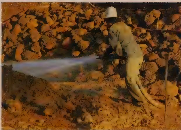
**Figure 12.126** A miner at Bo Rai, Trat Province, Thailand, uses a water cannon to force the ruby-bearing soil into the separation jig. (Photo: John Rouse, ca. 1983)
