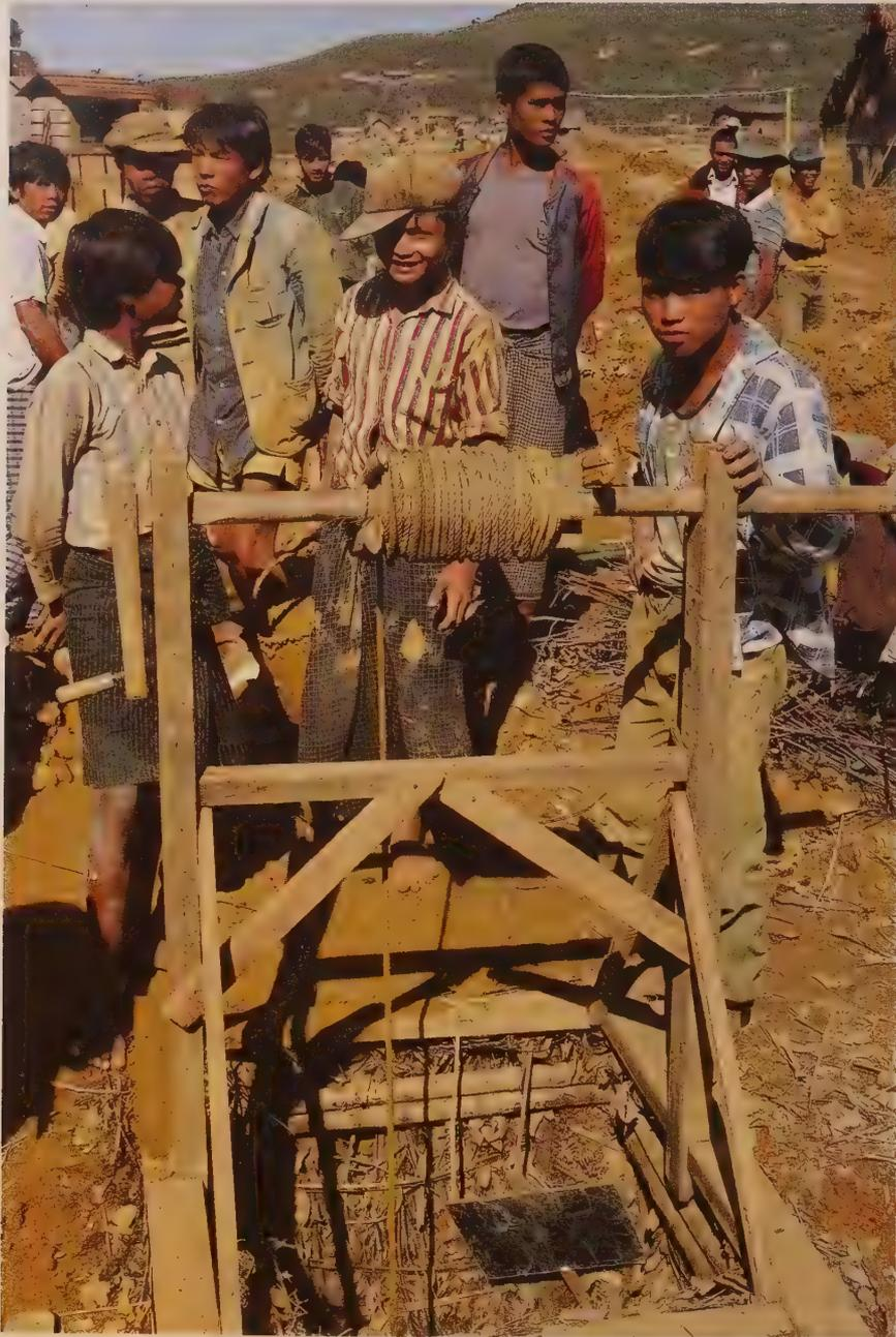
**Figure 12.40** Raising gravel from a *lebin* (square pit) at Mogok's Inn Gaung ('Big Hole Mine'). Note the foil reflector at the pit entrance, which is designed to direct light to the pit's bottom. (Photo: Thomas Frieden)
