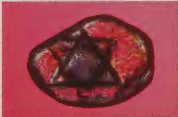
Figure 2.21 Corundum crystals often display raised triangles on the pinacoid face, resulting from oscillation between the rhombohedron and pinacoid. Such triangles are in opposite position on each end of the crystal. If the crystal is transparent and thin enough, the triangles create a “Star of David” effect, such as that shown above in a 2.5-ct Yogo (Montana) stone. (Photo: John Koivula/GIA)
