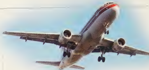
MODERN AIRCRAFT Light yet strong enough to bear great pressure, aluminium is ideal for aircraft bodies.
