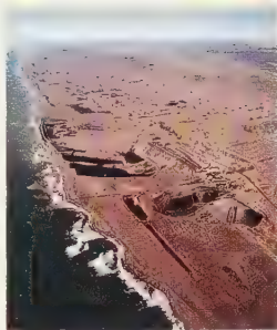
NAMIBIA Some beach deposits in Namibia are rich in alluvial diamonds. Huge earth-moving operations take place to remove the overlying sand to reach diamond concentrations on bedrock.
