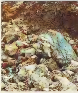
COPPER MINE, ZAMBIA Malachite and chrysocolla have formed as an alteration product of copper and are visible here on the surface of the Kansashi open-pit copper mine, Zambia.
