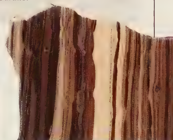
POLISHED OIL SHALE This polished section of oil shale shows darker, kerogen-rich layers. Darker colours come from the organic matter.
