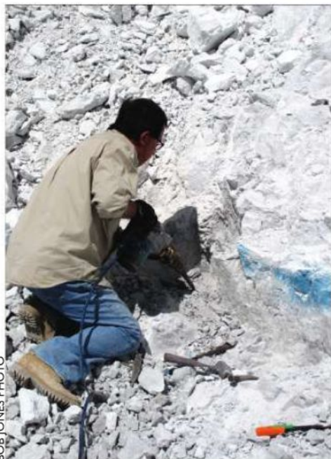
An electric power hammer reduced the boulders of hard rhyolite into manageable chunks for hand tools.
