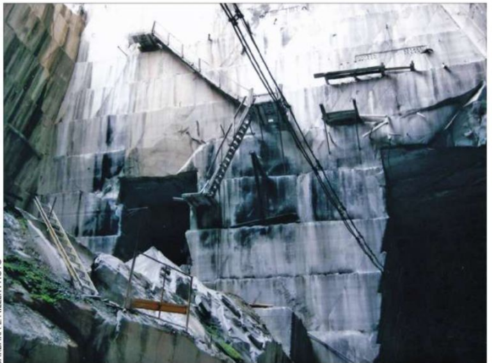
In the middle room of the subterranean quarry, the circa 1925 stairway is still attached to the wall and a large marble pillar supports the ceiling.
