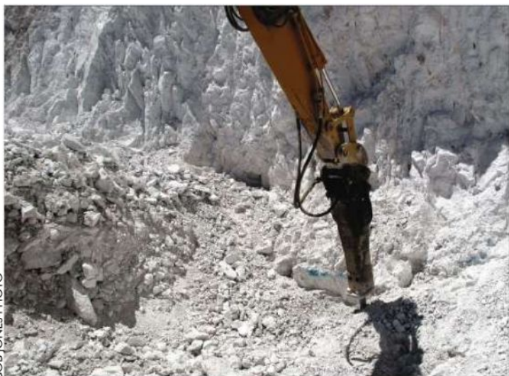
Clay uses a massive hydraulic hammer—actually a tapered point suspended from the arm of a backhoe—to crack the snow-white rhyolite into large boulders.
