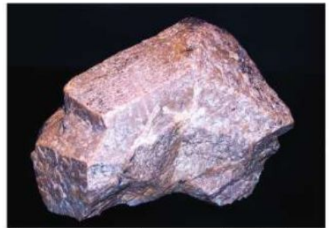
The slow cooling of the once very deep Continental Shield produced large crystals of many rock-forming minerals, such as feldspars.
