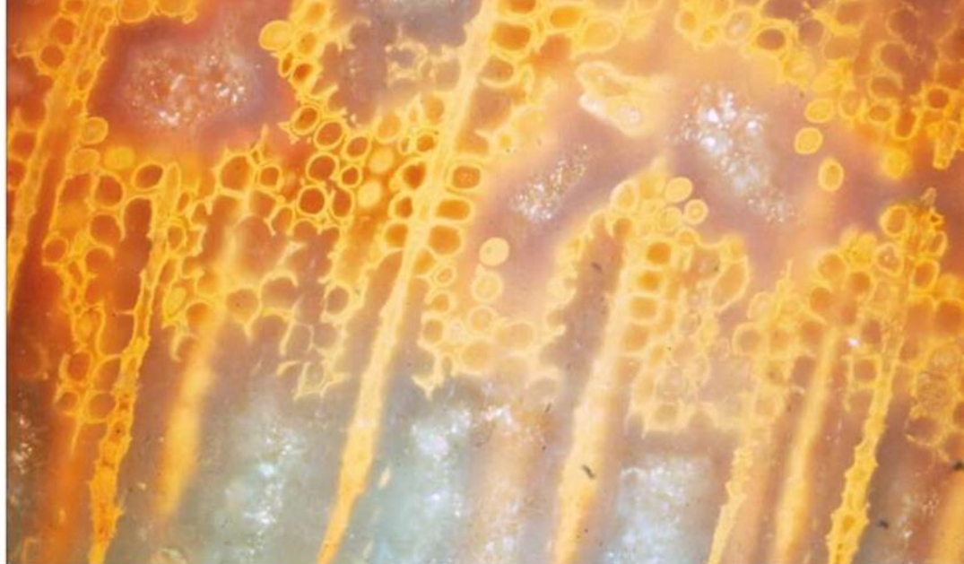
The silica-filled cells of the original wood are easy to see in this close up of an Arizona petrified wood slice.
