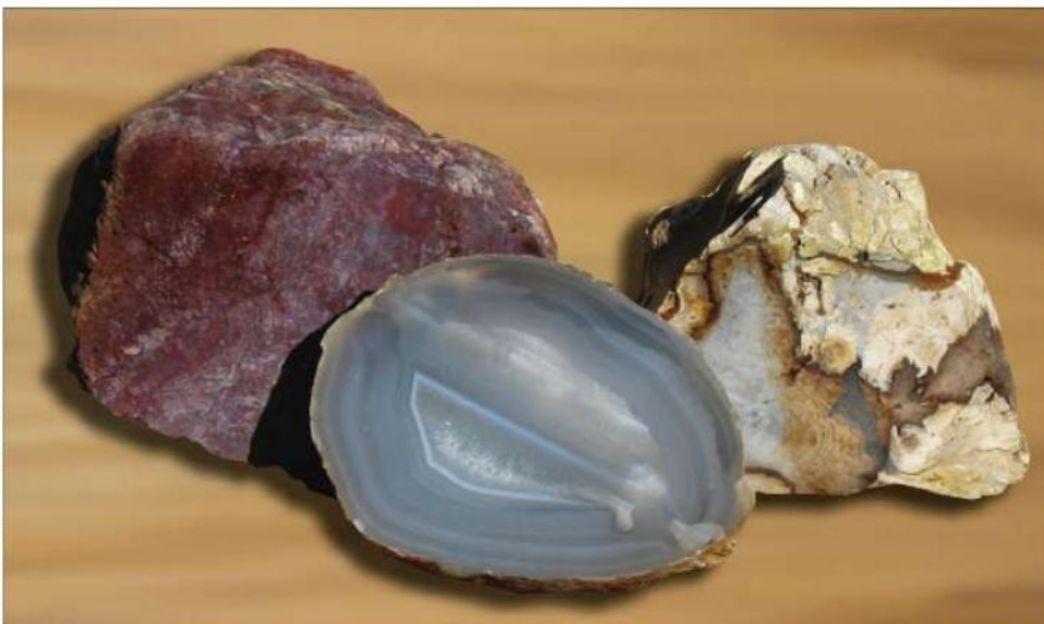
Dust from red jasper, Brazilian agate, and petrified wood all contain high amounts of silicon dioxide (SiO 2 ), which can cause silicosis when inhaled.
