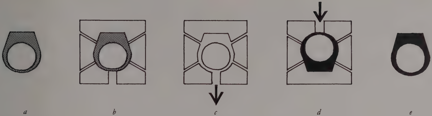
Fig. 19 The principle of lost-wax casting:
