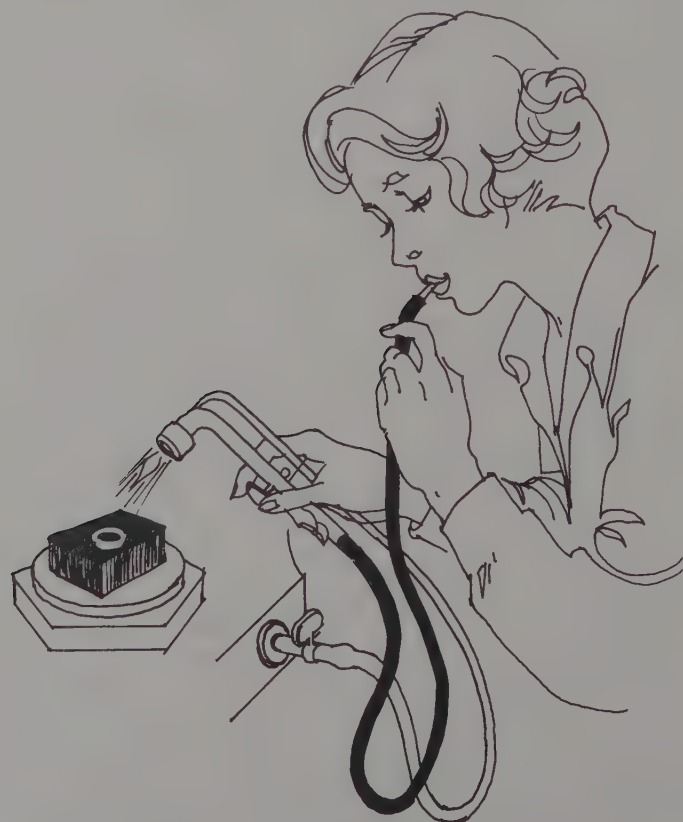
Fig. 18. Using the mouth blow torch, which employs a mixture of gas and mouth-blown air.
