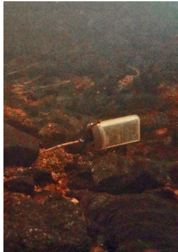
Figure 9. Temperature logger on the river bottom. Photo Paul Aspholm.
