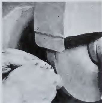
GRINDING AGATE TO SHAPE
