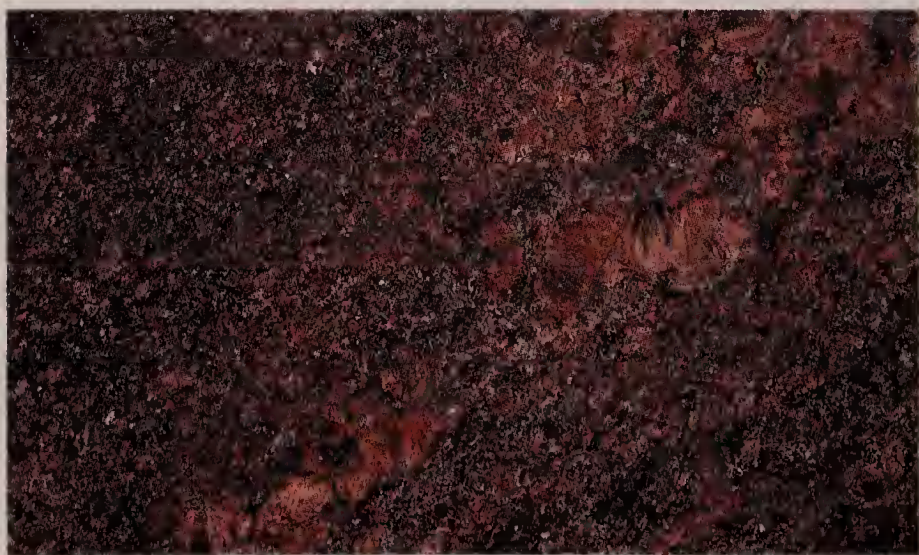
Hard granite makes an excellent building stone. Polished slabs form the facing of the Federal Building in Reno.
