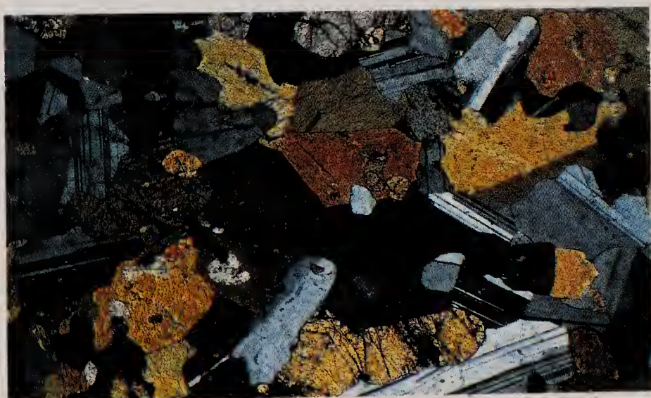
Thin section of feldspar grains in gabbro, as seen through a microscope.
