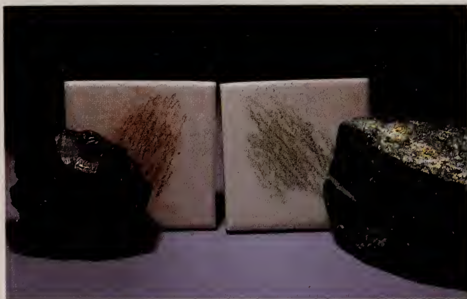
The streak colors of hematite, left, and malachite.
