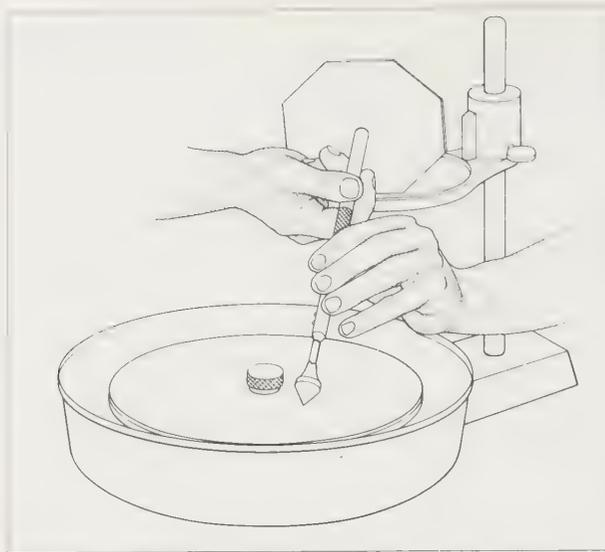
Far left: The jamb peg in use. The faceting angle may be varied simply by inserting the tip of the peg into a new hole
