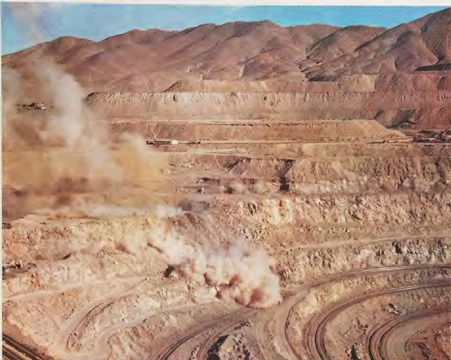
*Above: Blasting the terraced quarry faces of one of the world's largest copper workings, at Chuquicamata, Chile*
