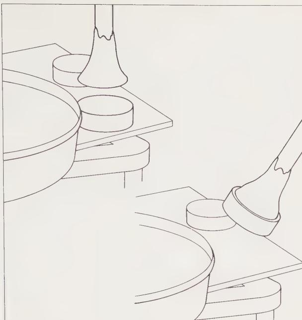
*Far right: Making sure that the dop stick and the stone are correctly aligned before the wax sets hard*
