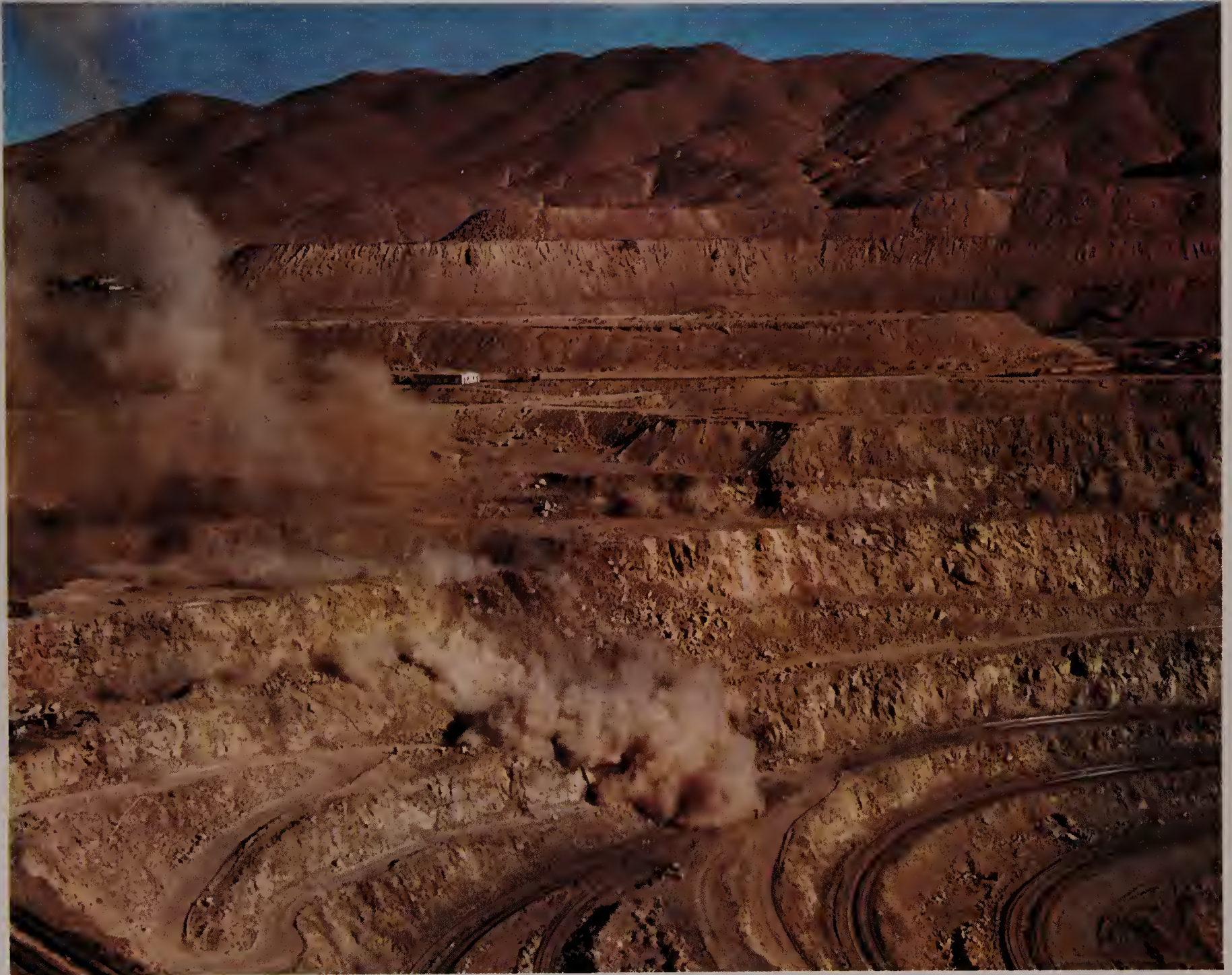
Above: Blasting the terraced quarry faces of one of the world's largest copper workings, at Chuquicamata, Chile
