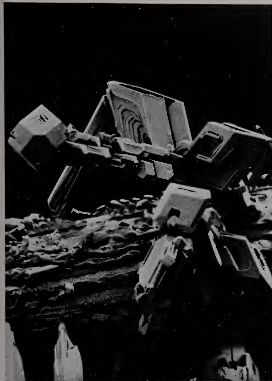
Above: Synthetic tungsten crystals seen under the electron microscope. These manmade crystals show sharp edges and smooth faces. Some crystals have a hollowed-out look, where growth has taken place fastest at the edges
