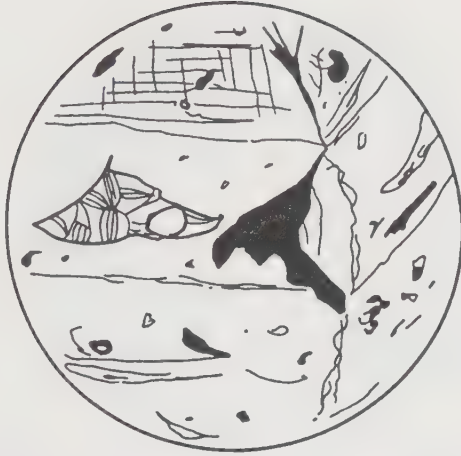
Figure 13.1 Two-phase inclusions and zoning in an alexandrite grown by the flux-melt method
