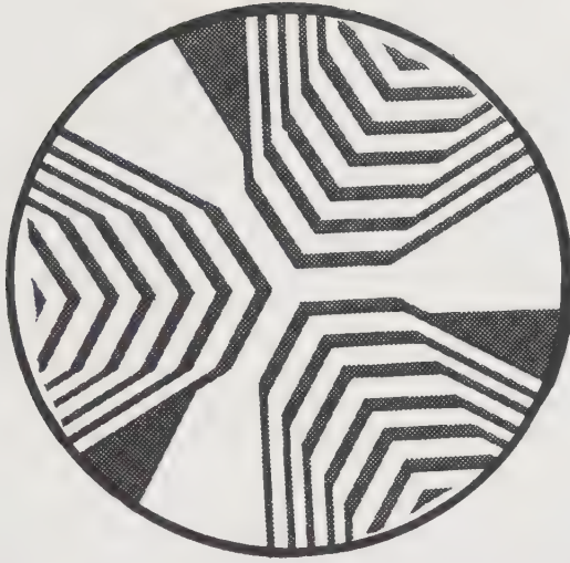
Figure 10.1 Natural quartz viewed between crossed polars and displaying twinning. (After P.G. Read)
