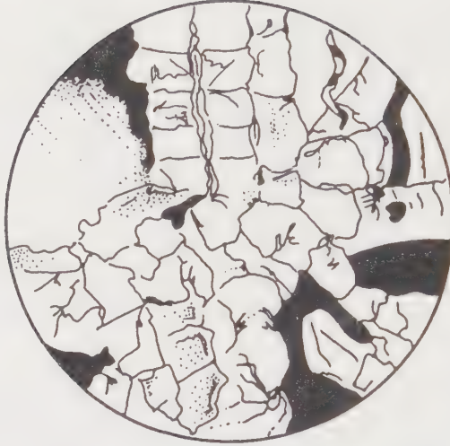
Figure 11.1 Characteristic hexagonal markings within a single colour patch in a synthetic opal
