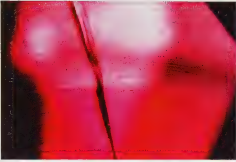
Plate 1 The classic Verneuil inclusion-curved growth lines in a synthetic ruby. This effect is not always easy to see, and careful positioning of the specimen may be needed
