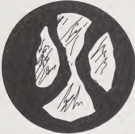
Figure 13.2 Anomalous double refraction of a spinel grown by the flame-fusion method, as seen between crossed polars
