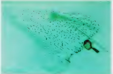
Plate 22 Droplets of flux accompany a crystal, probably phenakite, in a flux-grown emerald
