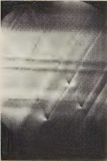
Fig. 10.4. The 'plato' effect in a small colourless synthetic sapphire taken between crossed nicols down its optic axis.
