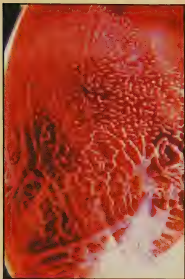
▲ 10. Chatham Ruby: Highly characteristic, lacelike 'feather' (fingerprint inclusion). 10x
