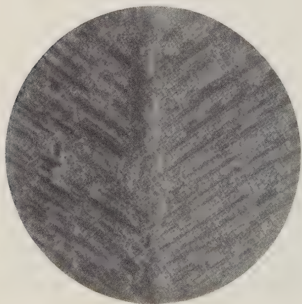
Fig. 2.3. Surface structure of a 'twin' boule of synthetic spinel. 15x
