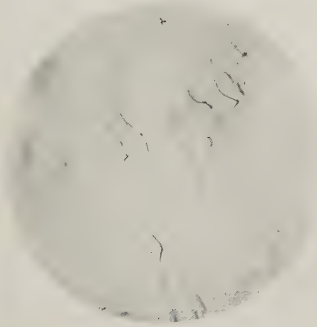
Fig. 14.6. Drawn-out bubbles in synthetic greenish-yellow spinel.
