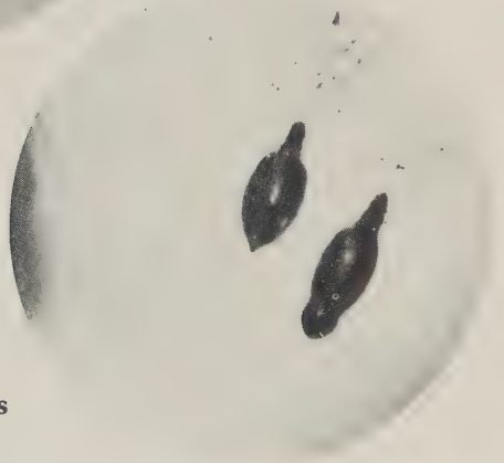
Fig. 10.6. Bomb-like bubbles with trails in a synthetic sapphire. Approx. 25x
