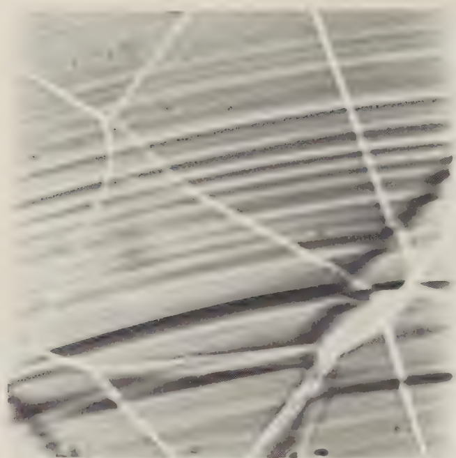
Fig. 14.1. (Above) Curved striae, characteristic of ruby red synthetic spinel.
