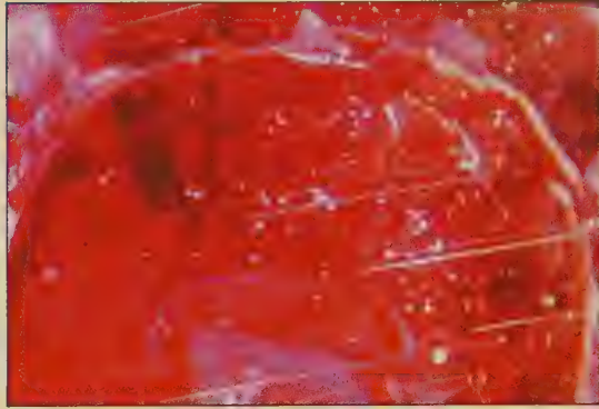
▲ 59. Doublet (imitating whole natural Ruby): Straight parallel lines (edges of polysynthetic twin lamellae) in the natural ruby crown; spherical air bubble in the cement layer above the synthetic ruby pavilion. 10x
