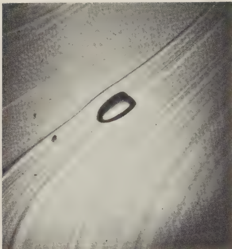
Fig. 21.1. A bullet-shaped bubble in a paste. 25x
