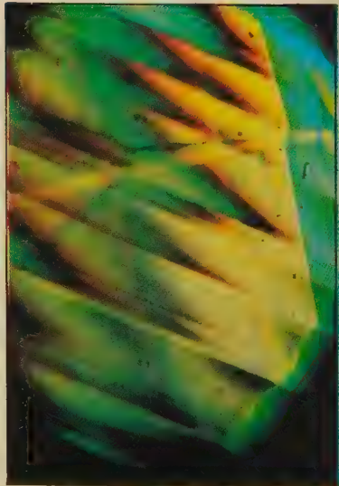
▼ 22. Verneuil Sapphire: The Plato-Sandmeier effect between crossed polars. 10x
