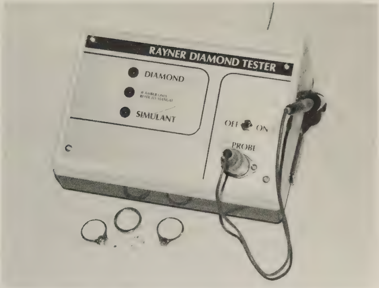
Fig. 8.7. The Rayner Diamond Tester which uses a thermal probe to identify diamonds.
