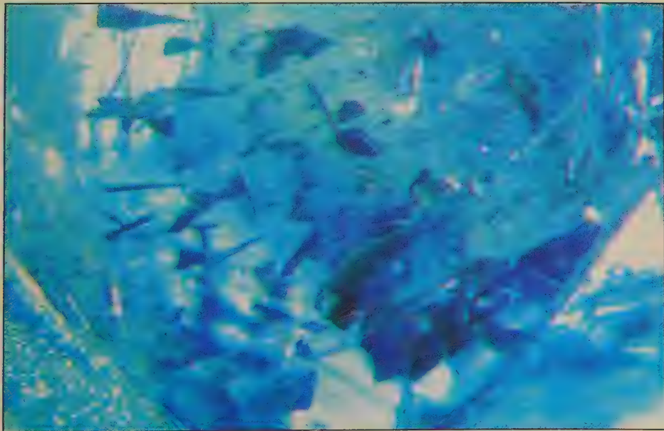
▼ 25. Chatham Sapphire: Concentration of typical platinum inclusions. 15x
