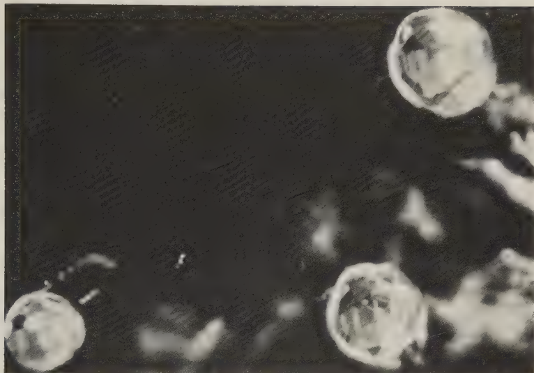
Fig. 2.14. Inclusions which have a natural appearance in synthetic spinel.
