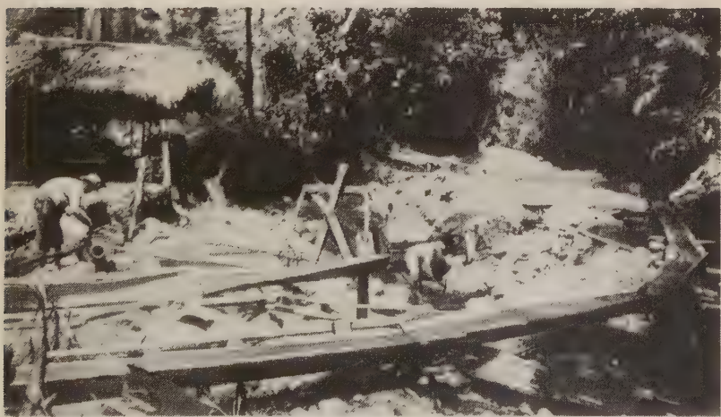
A PLACER GOLD MINE IN THE JUNGLES OF PANAMA. Note sluices in the foreground.
