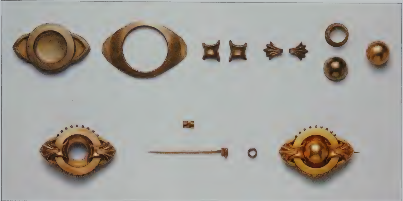
Demonstration model of a machine-made gold brooch with its component parts, made by T. & J. Bragg of
