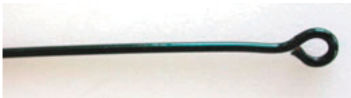
Figure 24 The Completed Eye Loop
