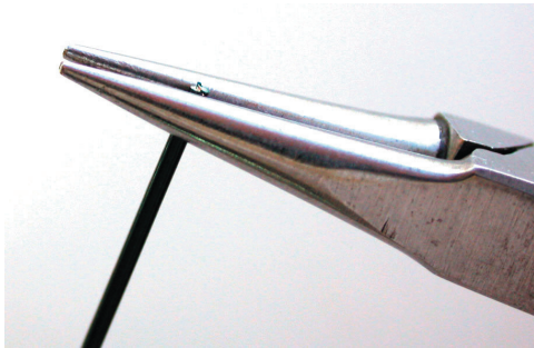
Figure 48 A, B, & C Making a P Loop Using Round Nose Pliers.
