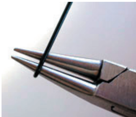
Figure 21A- Wrap the Wire Around the Pliers
