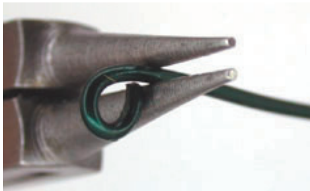
Figure 49 Grip the Wire Below the loop
