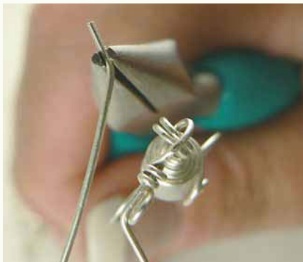
19 Use chain-nose (or flat-nose) pliers to bend up the last ¼" (6 mm) of wire, which makes it easier to run the ear hook into your pierced earlobe. Option: File the wire end with a flat file or use a cup-burr on a small handheld drill to smooth the wire end. This is especially important if you cut your wire with inexpensive cutters, which often leave burrs on the wire.
