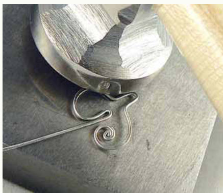
16 Use a chasing hammer to forge the outer edges of the heart shape, taking care to avoid other areas of the heart.
