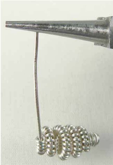
16 Grasp the base wire end in the round-nose pliers, about one-fourth of the way from the tips of the jaws. Notice that the bead is facing to the right. Wrap the wire around the lower jaw of the pliers by turning the tool away from you.
