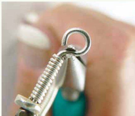
19 “Break the neck” using the tips of the chain-nose pliers.
