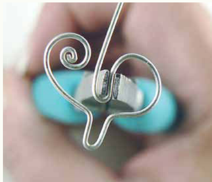
14 Bend the wire around and up, using the tool to shape the wire.
