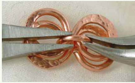
14 Close the jump ring securely using chain-nose or bent chain-nose and flat-nose pliers.
