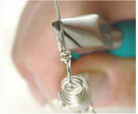
15 Grasp the long straight wire just a tiny bit above the spiral in chain-nose (or flat-nose) pliers.
