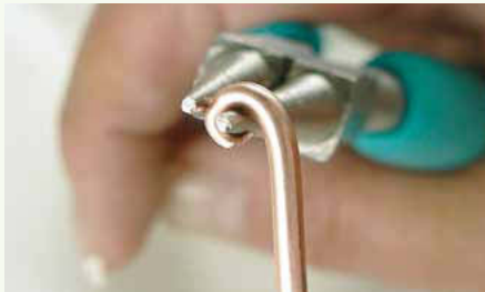
16 Use round-nose pliers to start a small spiral loop on each wire end.
