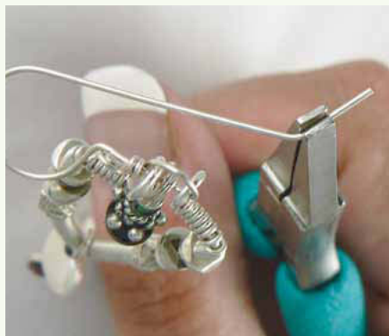
35 To finish, bend back the tail end of the ear hook. As an option, you may want to file the wire end to smooth the end. The ear hook also may be hammered with a plastic mallet to work-harden it.
