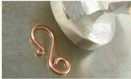
35 Lightly hammer the back of the hook shape with a chasing hammer.
