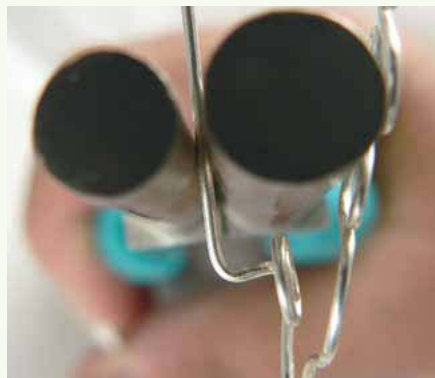
26 Take hold of the wire in the jaws of large bail-forming pliers.
