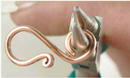
34 Use small round-nose pliers to bend another loop in the straight end of the wire.
