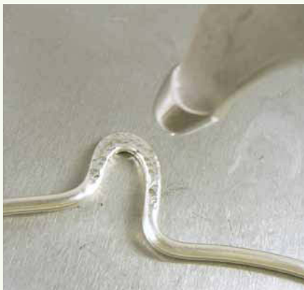
16 Use a small embossing hammer to texture the tip of the heart.
