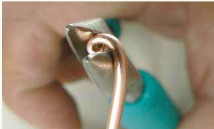
17 Use chain-nose (or flat-nose) pliers to tighten the beginning spiral.
