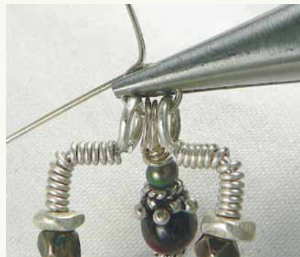
27 Close the loop sideways, pressing firmly.
