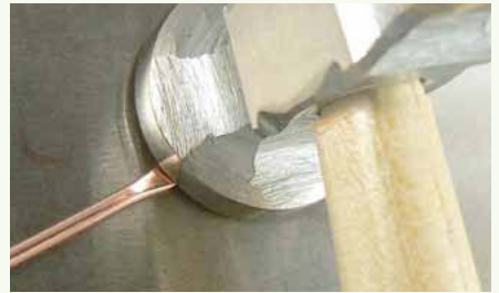
15 Hammer each wire end separately on a small steel bench block.
