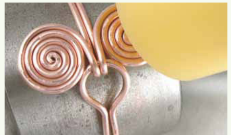
21 Hammer the bangle gently with a hard-plastic mallet.
