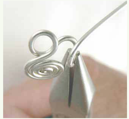
12 Before spiraling in the other wire end, open up its loop sideways using either chain-nose or flat-nose pliers.
