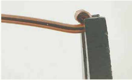
31 Spiral in the wire just a tiny bit.
