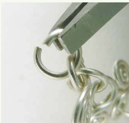
28 Open the second jump ring sideways and run it through the top loop on the middle shaped wire link.
