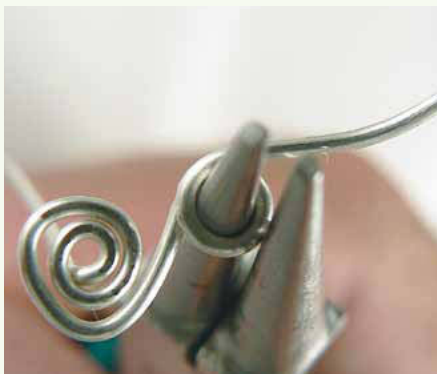
34 Continue bending the wire around to form a tiny decorative loop.
