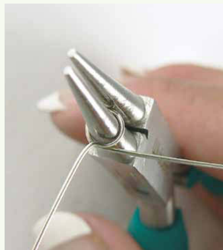
24 Flush-cut two pieces of 22-gauge wire, each 3" (7.5 cm) long. Pick up each piece separately and make eye-pin loops (see the Basic Techniques section). Stop before wrapping the loops.
