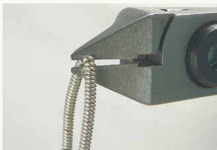
7 Cut the coil at the bend.
