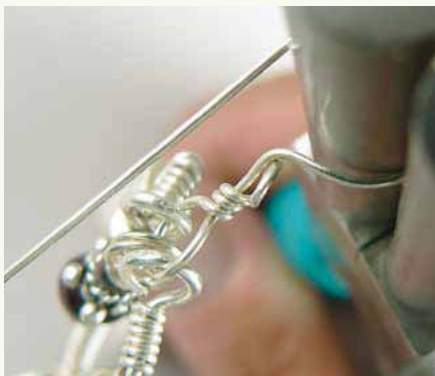
34 Bend the wire over the tool to form a shepherd's hook shape.
