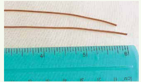
21 Clean and flush-cut two 6" (15 cm) pieces of 16-gauge wire.
