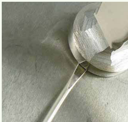
17 Use a chasing hammer and bench block to forge one end of the heart-shaped wire.
