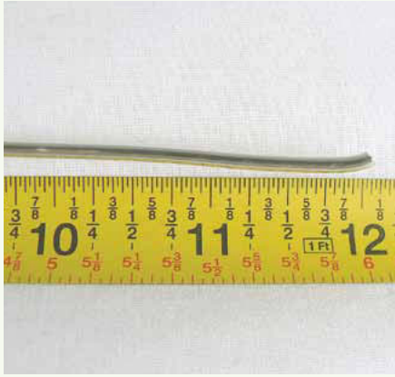
10 Flush-cut 1' (30.5 cm) of 10-gauge wire.
