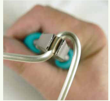
12 Using flat-nose pliers, bend the wire to the side, against the edge of the pliers.
