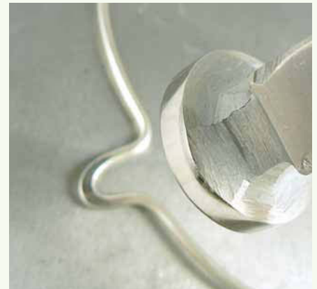
15 Using a chasing hammer and a 4" x 4" (10 x 10 cm) square steel bench block, hammer the tip of the heart. Don't overdo this step; the objective is to flatten the wire a bit, but not to thin it down too much.
