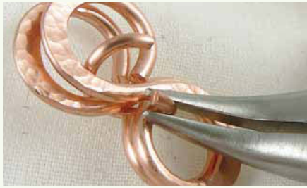
13 Run the jump ring through the midsection of both figure-eight links as shown.
