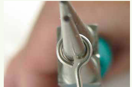
21 Reinsert the round-nose pliers into the loop and rock it forward until it resembles a lollipop.
