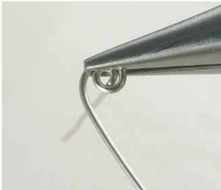
31 Spiral the wire around loosely as shown.
