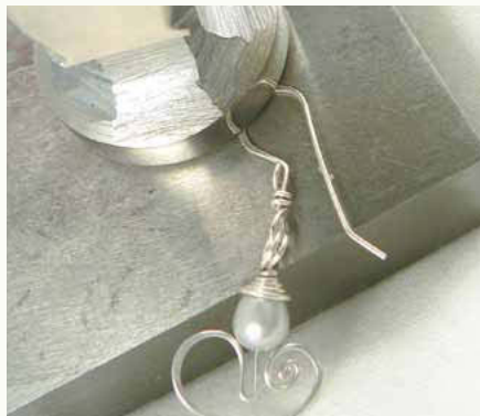
20 Option: Hammer the rounded portion of the ear hook on a small steel bench block, using a chasing hammer with a slightly convex face. Take care to hammer the wire lightly, as you don't want to thin down the wire too much.
