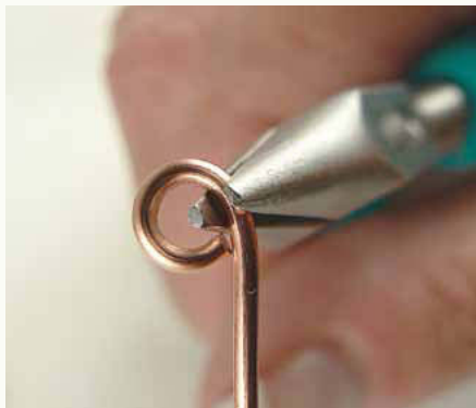
13 Switch to chain-nose pliers. Grasp the wire inside the loop, right where the wire end touches itself.
