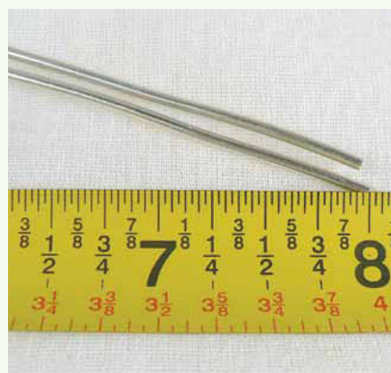
24 Measure and flush-cut two 8" (20.5 cm) lengths of 14-gauge wire.
