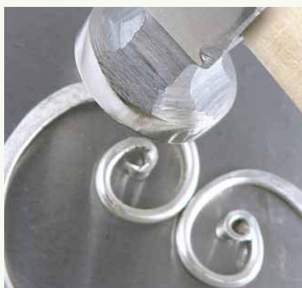
23 Switch to a chasing hammer and, placing the top portion of the heart-shaped wire on a 4" x 4" (10 x 10 cm) size steel bench block, hammer just the outer edges of the heart. Switch to a small embossing hammer and use it to texture the flattened areas of the heart-shaped wire.
