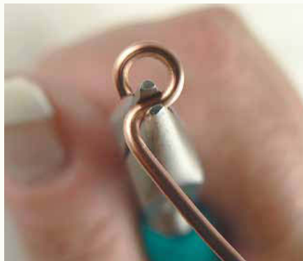
14 Bend the wire straight back against the edge of the tool.
