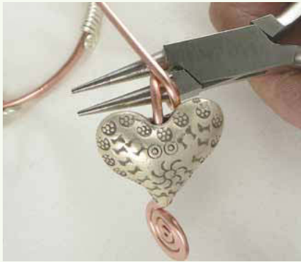
36 Wrap a loop on the back of the small round-nose pliers.
