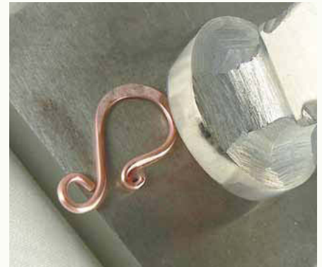
18 Hammer the back of the hook shape to flare it out a bit (don't overdo this step), and the hook is finished. File it if necessary to remove any tool marks.
