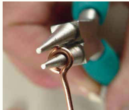
15 Reinsert the round-nose pliers and straighten out the wire so that it resembles a lollipop.
