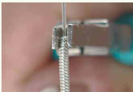
4 Press down the coil ends very firmly with flat-nose (or chain-nose) pliers.
