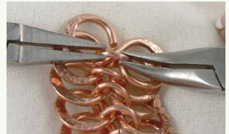
18 Continue connecting figure-eight links to one another in the same pattern. Close all jump rings very securely.
