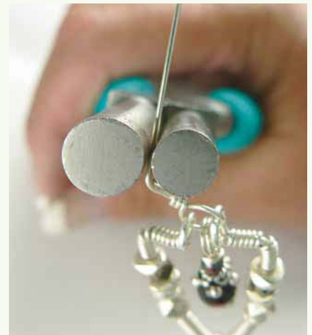
33 Grasp the wire with either large bail-forming pliers (shown) or large round-nose pliers.
