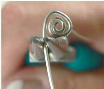
32 Grasp the wire in a new position, in the middle of the round-nose pliers.
