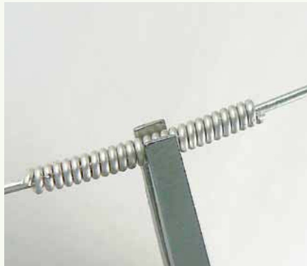
11 Grasp a coiled wire piece in flat-nose pliers, just to the right of center.
