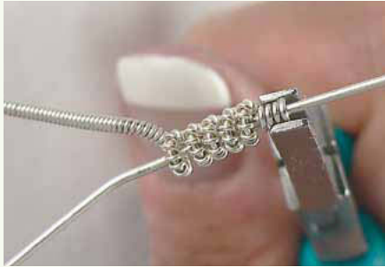
16 Coil the entire length of wire and press down the ends with flat-nose pliers as in Step 4.
