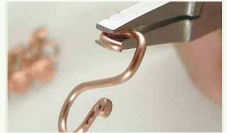
36 Open the hook's bottom loop sideways.
