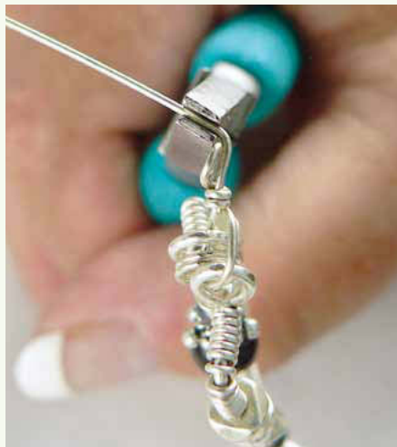
32 Using flat-nose pliers, bend the straight wire over the spiral.
