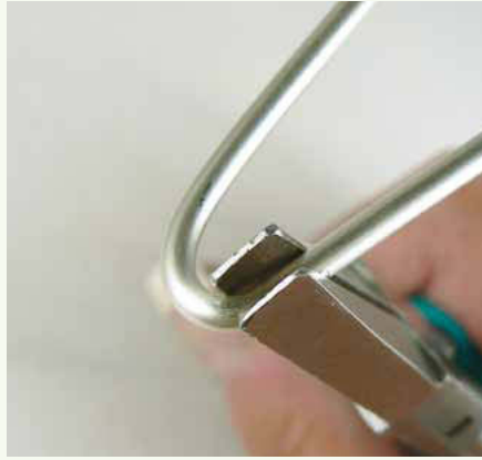
11 Using flat-nose pliers, bend the 10-gauge wire in half.
