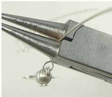
17 Place the wire in the back of large round-nose pliers right up against (but not inside) the box-joint on the tool. The wire should be pointing toward you.
