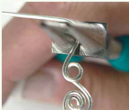
35 Grasp the wire in the back of the round-nose pliers in order to bend the wire in a new direction.
