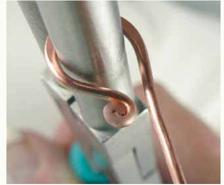
15 Bend the wire up and over until it touches itself, forming a hook shape.
