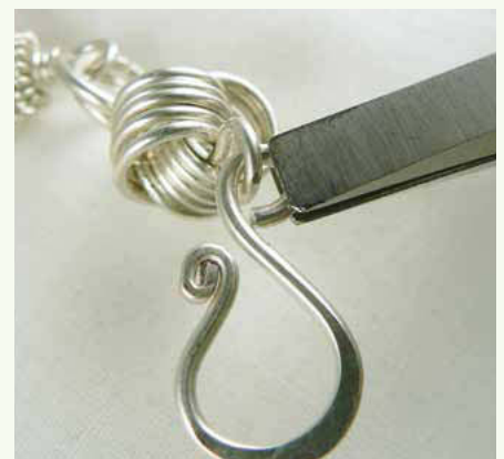
53 Be sure to close the eye-pin loop securely.
