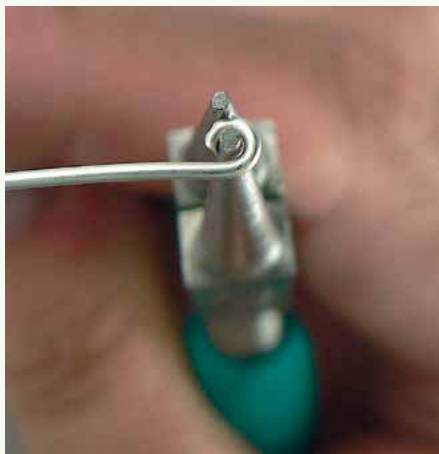
40 Start a small spiral in the end of the wire, using the tips of the small round-nose pliers as before.
