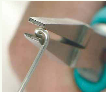
20 Use flat-nose (or chain-nose) pliers to tighten down the beginning spiral.
