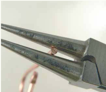
16 Place the straight wire end in the middle of the small round-nose pliers.
