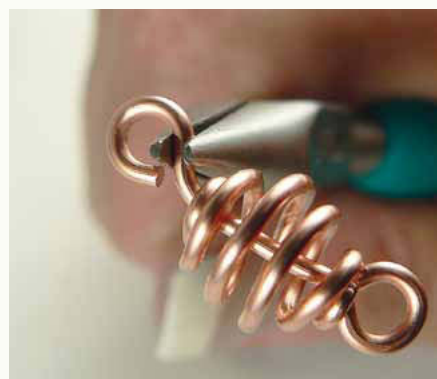
18 “Break the neck” as before, using chain-nose pliers and switch to round-nose pliers to straighten the loop on the wire.
