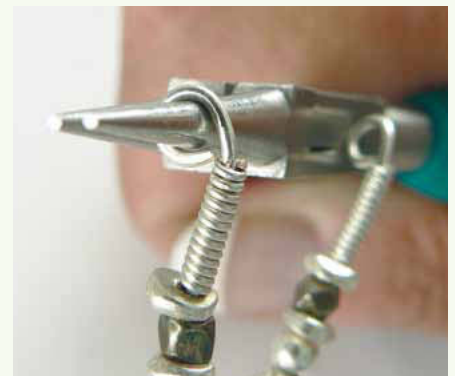
18 Bend small loops with the bare wire ends, in the middle of the small round-nose pliers. Note that each loop is facing the same direction.
