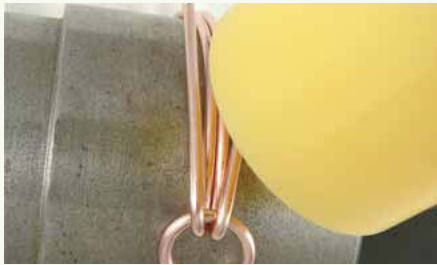
14 Hammer the wires gently with a hard-plastic mallet.
