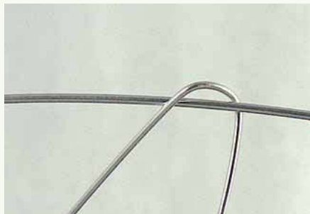
2 Flush-cut 2' (61 cm) of 26-gauge wire and bend it in half over a length of 24-gauge wire.
