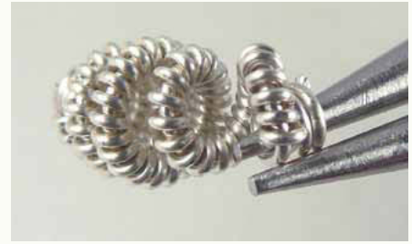
18 Remove the round-nose pliers, turn them around, and reinsert them into the coiled wire from the opposite end.
