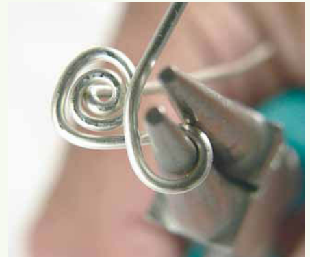
33 Bend a loop in the wire by wrapping it tightly around the tool.
