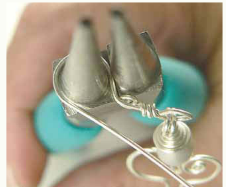
18 Use your fingers to bend the wire firmly around the tool, forming an ear hook-shape.
