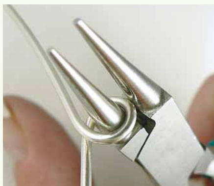
26 Wrap the wire around the back of the pliers, forming a loop.
