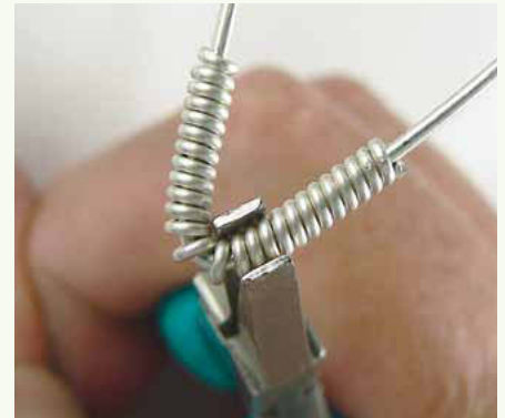
12 Bend the wire at a sharp angle as shown.
