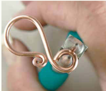
17 Bend the wire up and over until it touches itself, forming a loop.
