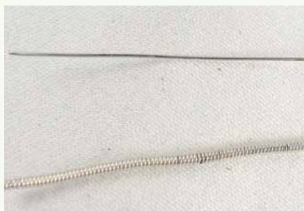
5 Remove the coil from the 24-gauge wire.
