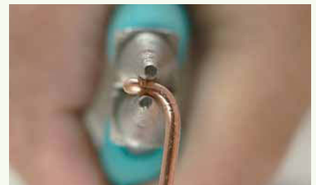
24 Bend the bent end of each wire piece forward using the tips of the round-nose pliers.
