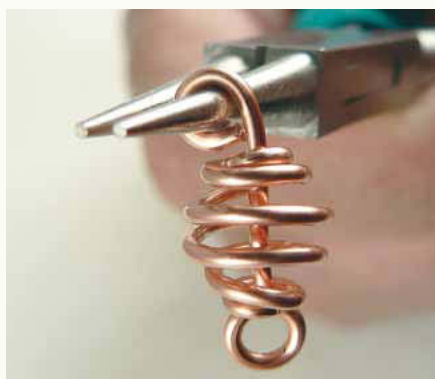
17 Bend the wire over in the middle of the round-nose pliers.
