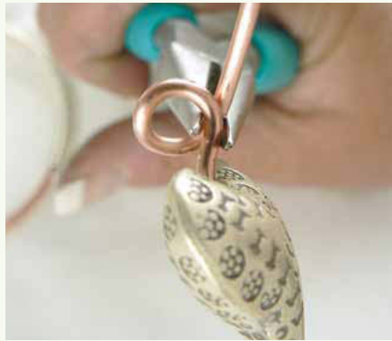
37 "Break the neck" using chain-nose pliers.
