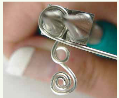
36 Continue bending the wire around the tool.
