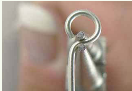
20 Use the tips of the round-nose (or chain-nose) pliers to bend the wire back sharply; this is known as "breaking the neck."
