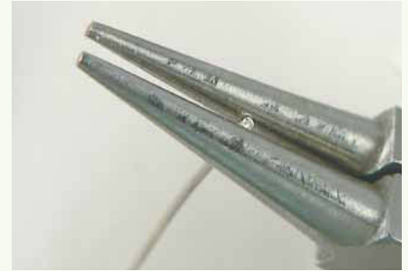
18 Place one end of the 20-gauge wire in the middle of the small round-nose pliers.
