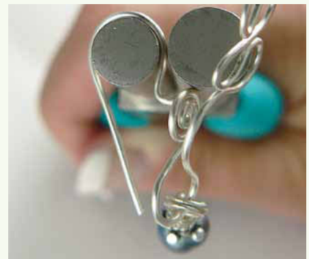
27 Use the smaller (6.8 mm) jaw of the bail-forming pliers to form the ear wire. Press the wire firmly against the tool with your fingertips.
