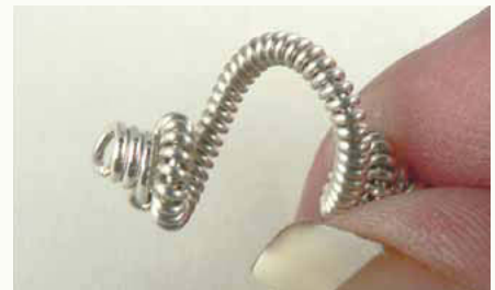
20 To insert a bead, first twist the coiled wire open with your fingers.
