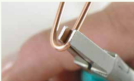
22 Bend the wire in half using flat-nose pliers.
