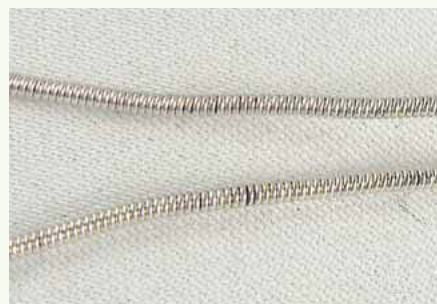
6 Bend the coil precisely in half.
