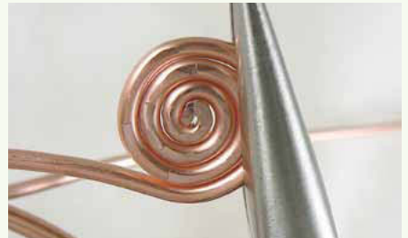
18 Spiral in the wire end using either chain-nose or flat-nose pliers.
