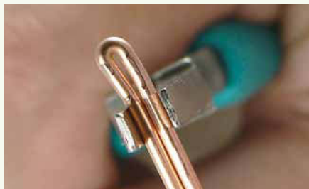
23 Use flat-nose pliers to press the wires closely together.
