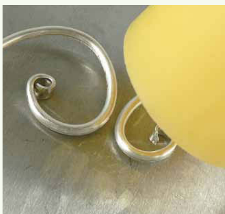
22 Use a hard-plastic mallet to hammer the top half of the heart.
