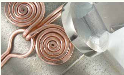
22 Use a chasing hammer to flatten the outer edges of both spirals on the bracelet mandrel. Then remove the bangle from the mandrel.
