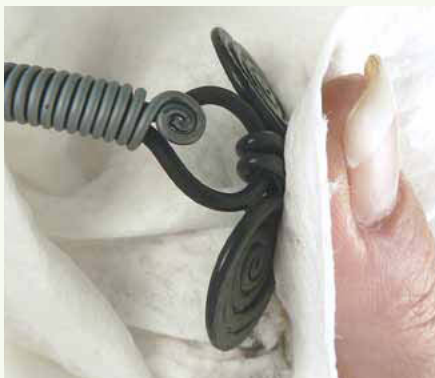
42 Dry the bangle thoroughly with a paper towel and polish it with 0000 (superfine) steel wool. Finish with jewelry polishing cloths.
