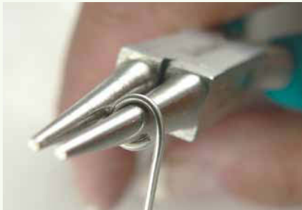
19 Bend the wire over in a loop as shown, ensuring that the wire touches itself.
