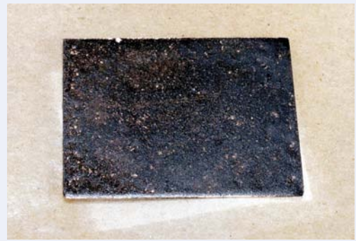
The copper with two coats of sealer
