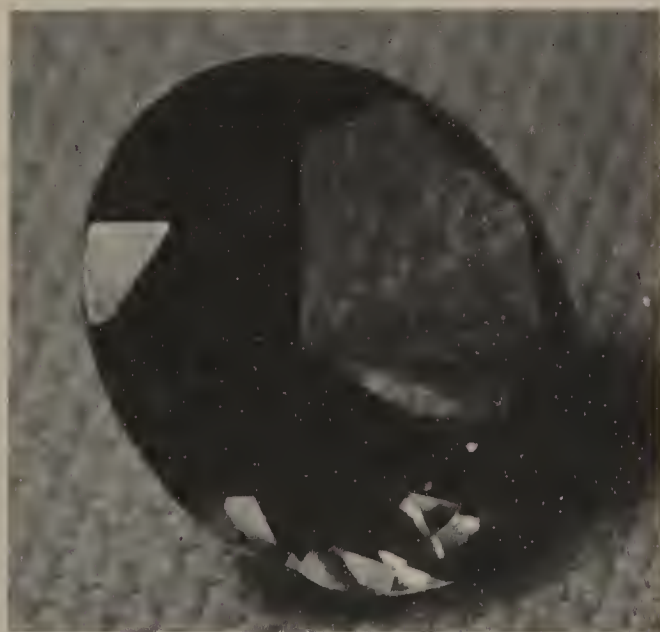
Another crown facet in a semi-finished state. With the final polishing of the main facets, the girdle facet will lose its four-sided appearance and assume its required three-sided shape.
