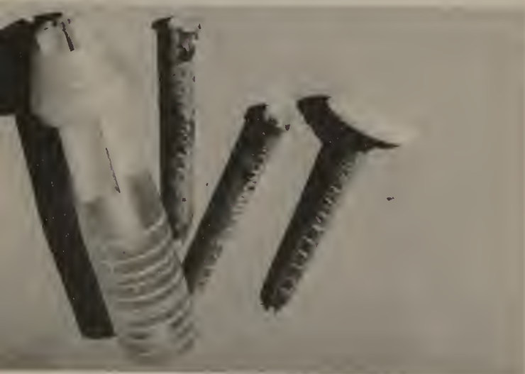
Metal dopsticks and holder suitable for all jobs but with particular suitability for opal.
