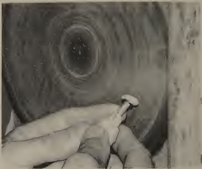
Sanding on a coated abrasive cloth disc (silicon carbide). This operation is carried out wet. The abrasive disc is attached to the supporting rubber back with a special disc cement.
