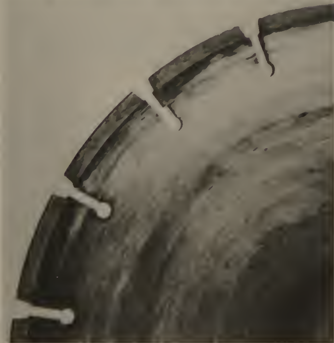
A segmental diamond saw blade. This particular blade has deep gullets to aid clearance of debris. It is used on a machine cutting soft materials.
