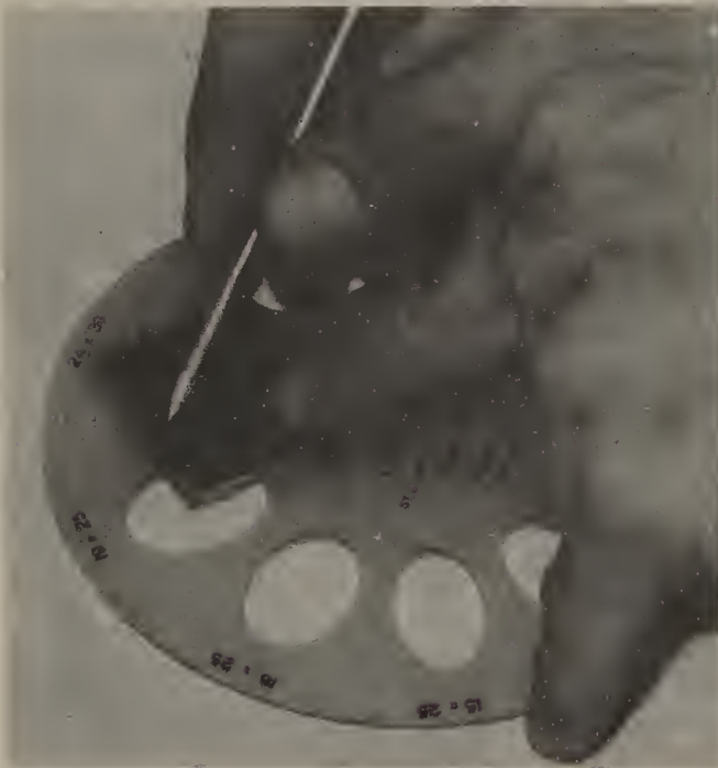
The metal pencil must be kept closely against the template opening to ensure accurate marking out.
