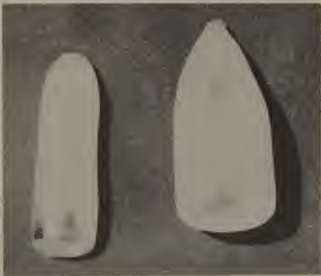
Typical synthetic boules. The left-hand one is a half-boule of clear corundum and that on the right is a full boule of white spinel.
