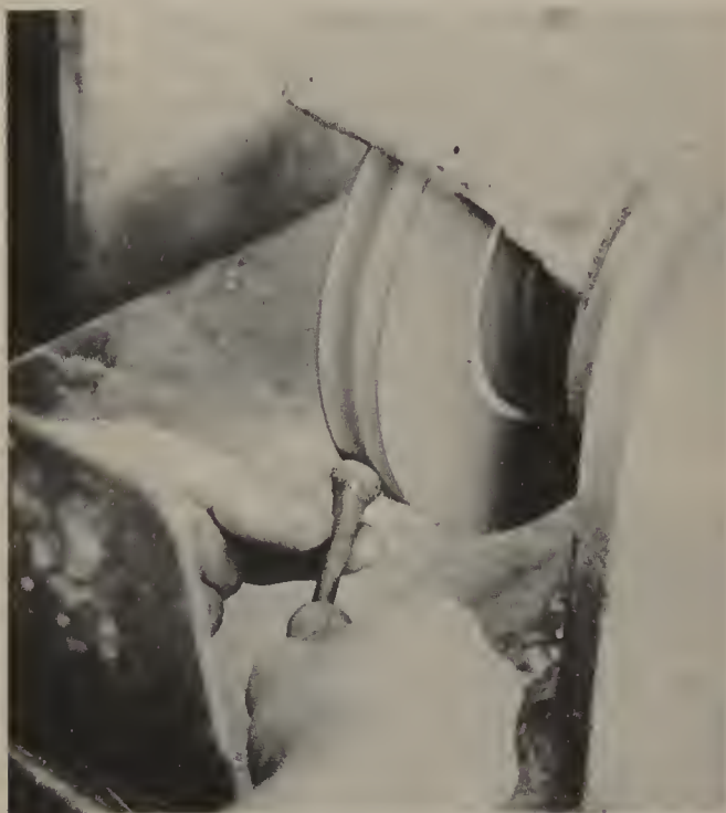
A profiled grinding wheel in use to shape the upper curve of a dopped stone. Note the position of the hands when holding the dopstick.
