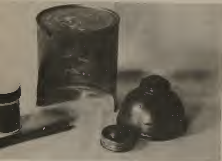
Dopping equipment: dop stove, powdered and stick wax and a metal spirit lamp.
