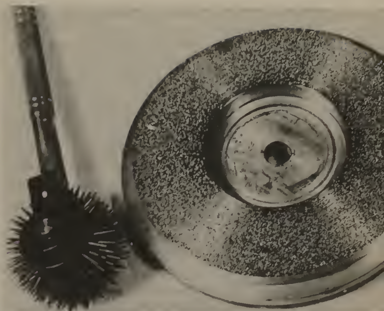
Lap scoring. An alternative method of preparing the soft metal lap for charging is by the use of a stippling wheel. A typical tin-type metal lap ready for its diamond charge is shown together with the wheel.
