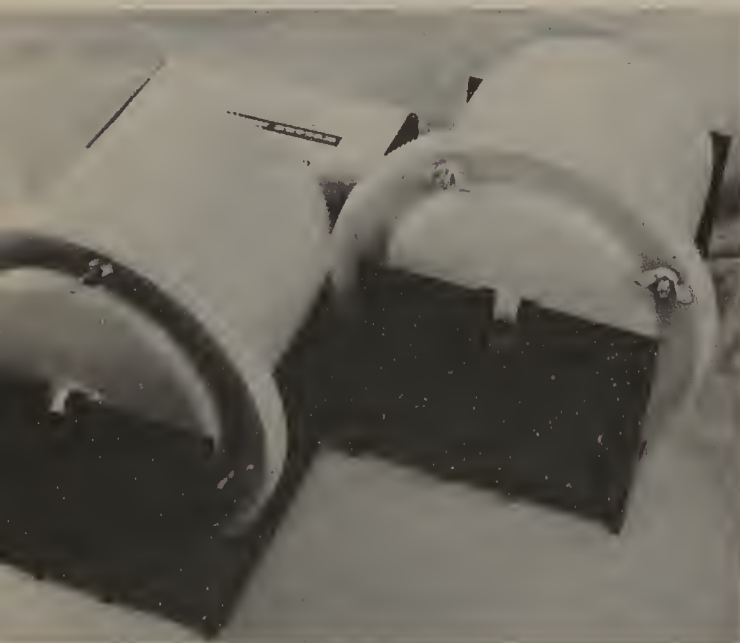
An ingenious tiny tumbler which has gear teeth formed on both edges of the barrel. These can be engaged with other barrels to enable up to five batches to be processed with a single powered unit. The capacity of such a string is approximately 500 g per barrel.
