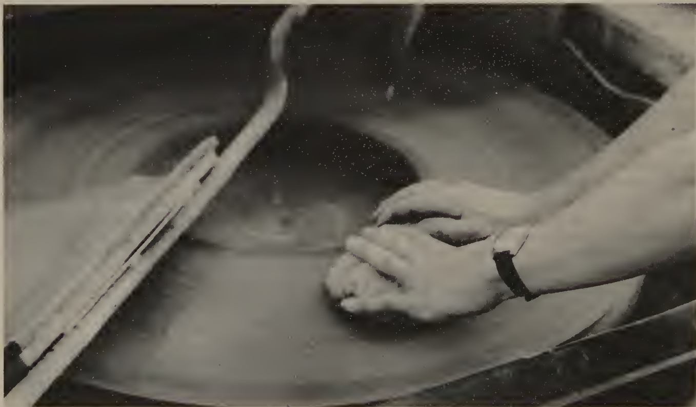
Hand lapping a sawn agate geode half on a large cast-iron flat lap using silicon carbide abrasive and water. This process is followed by fine grinding and then polishing on the vibrating lap.
