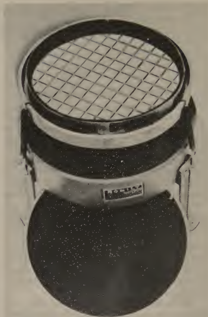
A vibrating lap attachment for the 'gemmaker' horizontal-type all-purpose machine to which it is shown fitted. The dark disc below is the polishing pad. (Photo by courtesy of Rytime Robilt Pty Ltd, Melbourne.)
