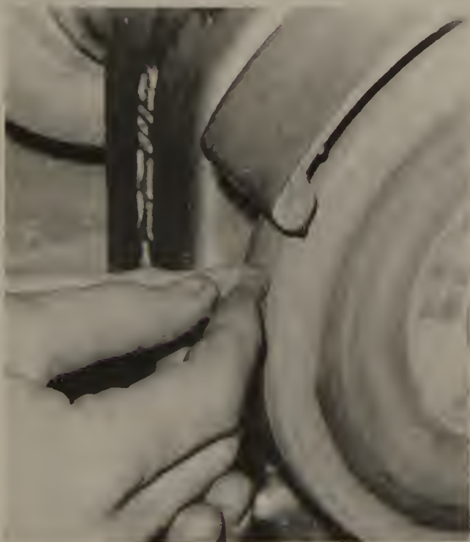
A cab preform being edge-ground on a silicon carbide wheel. The hold on the stone must be secure and the position of the fingers is shown.
