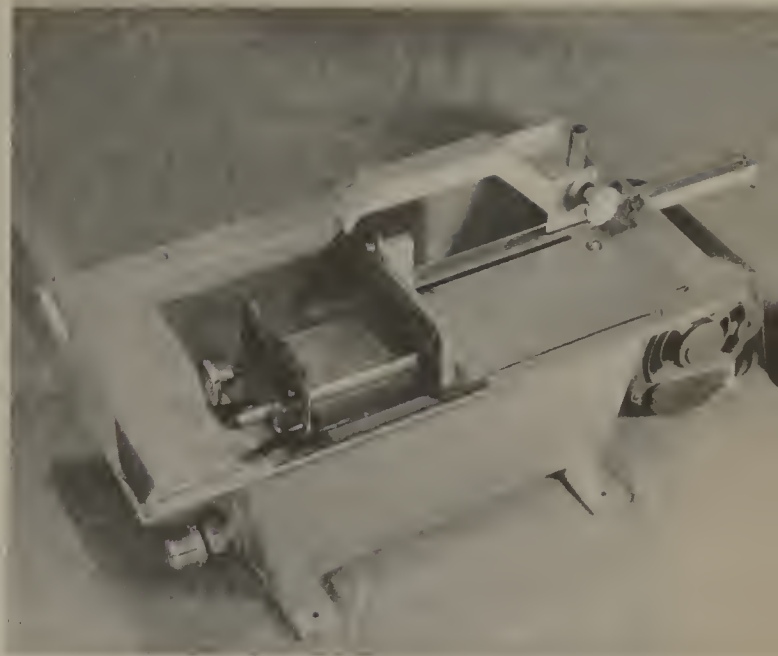
A trim/slab saw machine with vice and weight feed. This unit is designed to accept diamond blades from 150 mm to 250 mm in diameter. (Photo by courtesy of Halls, Cairns, Queensland).
