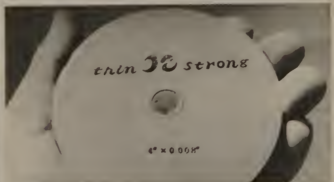
One of the ultra-thin continuous-rim diamond saw blades which is 100 mm in diameter and 0.2 mm thick. This particular blade is very good for opal cutting or faceting.
