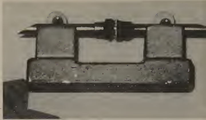
The waxed dopstick pressed into contact with the finished face of the stone in preparation for redopping. Note the angled end of the stick which ensures correct orientation of the stone when replaced in the head of this particular faceting machine.
