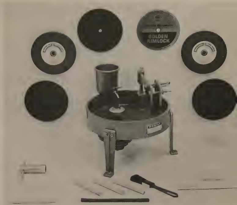
A horizontal-type 'gemmaker' all-purpose machine. The swinging arm fitted to the post on the side of the bowl is the holding device for sawing with a diamond blade on the vertical spindle. Attachments are supplied by the manufacturer which convert the base unit into a very good faceting machine.
