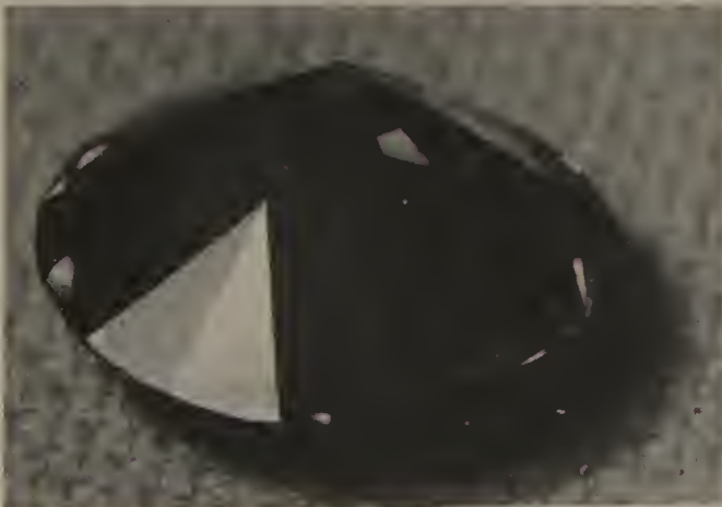
The overcut corrected to bring the junction between the two facets to a point.
