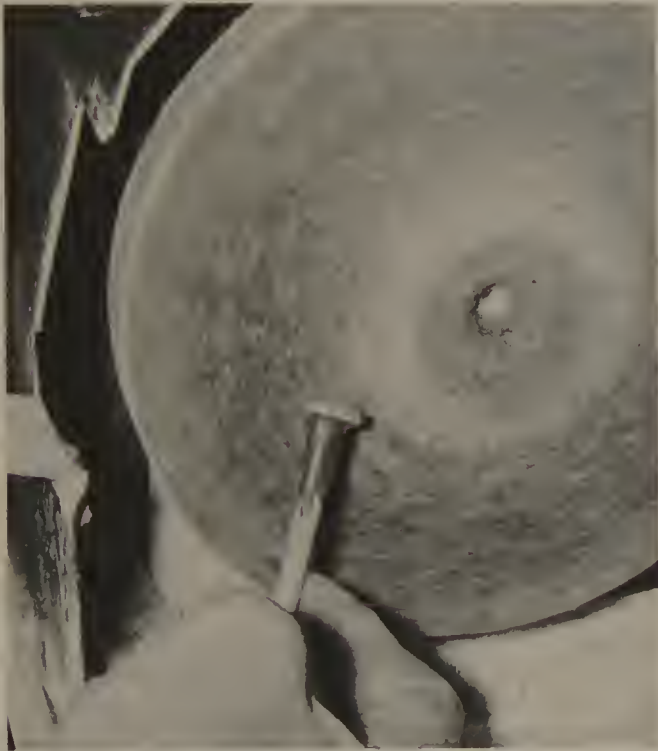
Prepolishing with pumice on a felt wheel.
