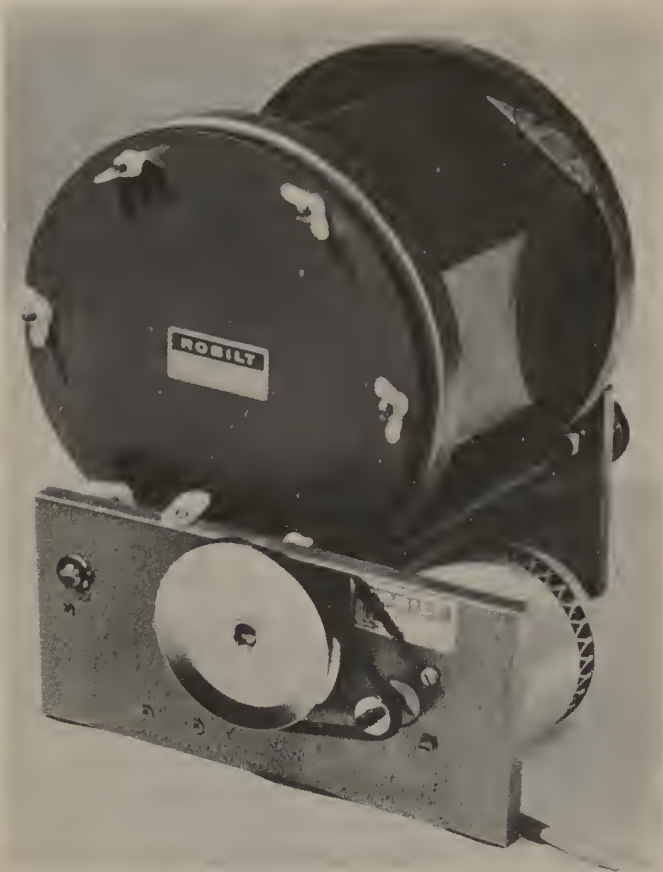
Convenient self-contained roller-type tumbling machine with a 4-litre octagonal rubber-lined barrel. (Photo by courtesy of Rytime Robilt Pty Ltd, Melbourne.)
