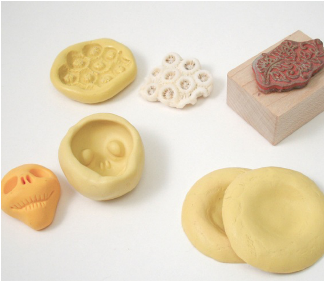
From left to right: Mold of a clay model skull for making reproductions; mold of a piece of coral; a rubber stamp; and silicone rubber baking supports created out of mold putty and used to support flowers.
