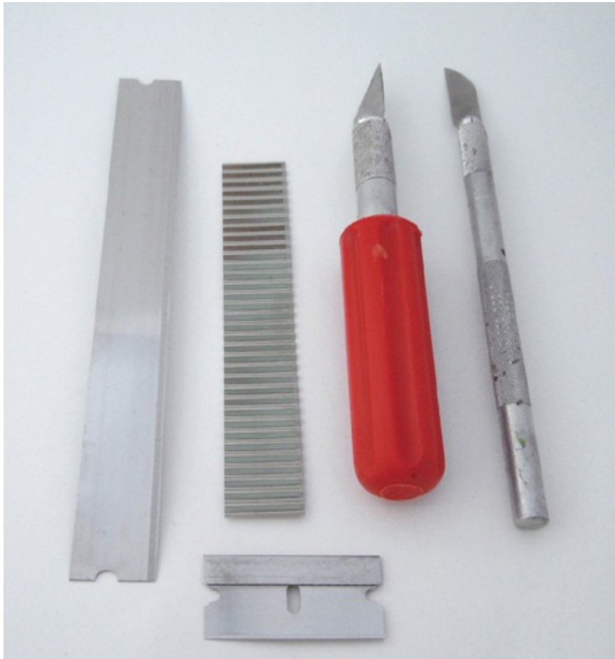
From left to right: Tissue blade, specialty blade, craft knife, X-Acto knife, single-edge razor blade
