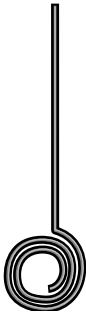
Figure 10-2: Coil the end of the wire to help keep the lampwork bead in place.
