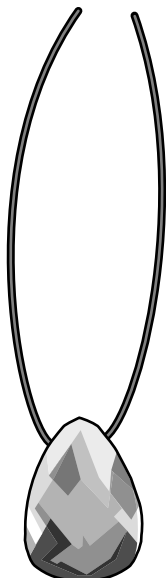
Figure 9-12: Bend both ends of the wire up toward the top of the teardrop.
