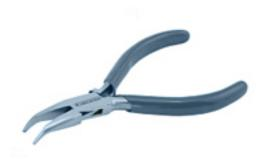
Above is an example of a pair of Beadalon Bent Chain Nose Pliers.
