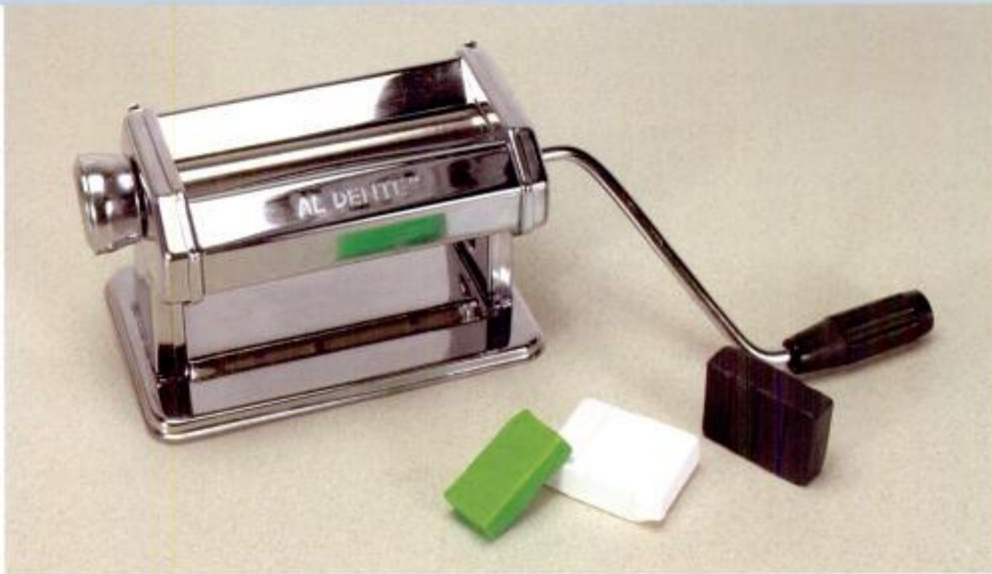
Clay can be rolled through a hand-cranked pasta machine like the one shown above to further condition it and to roll it into sheets in various thicknesses.
