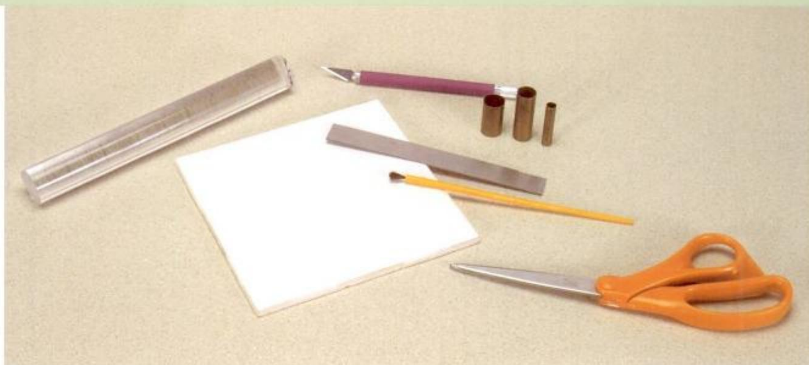
The tools shown above are used to cut, shape and pierce polymer clay. Clockwise from top left: acrylic roller, craft knife, circle cutters, tissue blade, craft paintbrush with plastic handle, ceramic tile and craft scissors.
