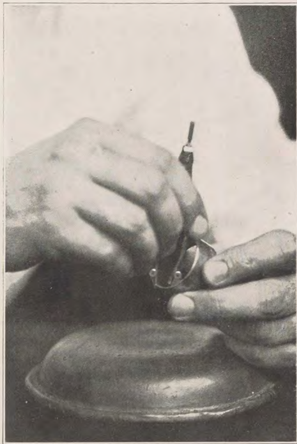
Drawing Lines on Inside of Napkin Rings, Using Small Piece of Rubber Instead of Lead in Dividers
