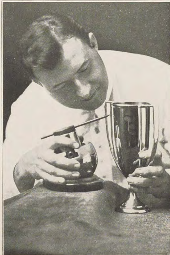
Method Used in Drawing Lines for Inscription Work for Loving Cups, Etc., Using Rubber Marker to Keep from Scratching
