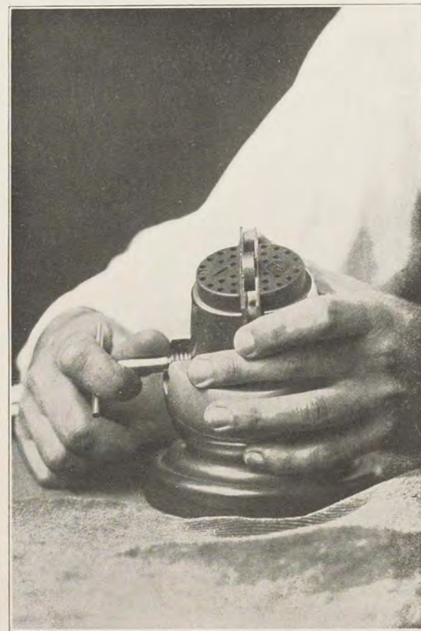
Correct Way of Holding Any Ring Between Two Strips of Lead, for Outside Ring Engraving
