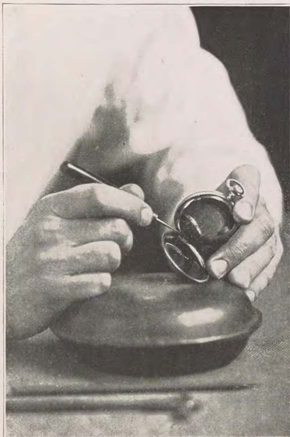
Replacing Pin After Engraving
