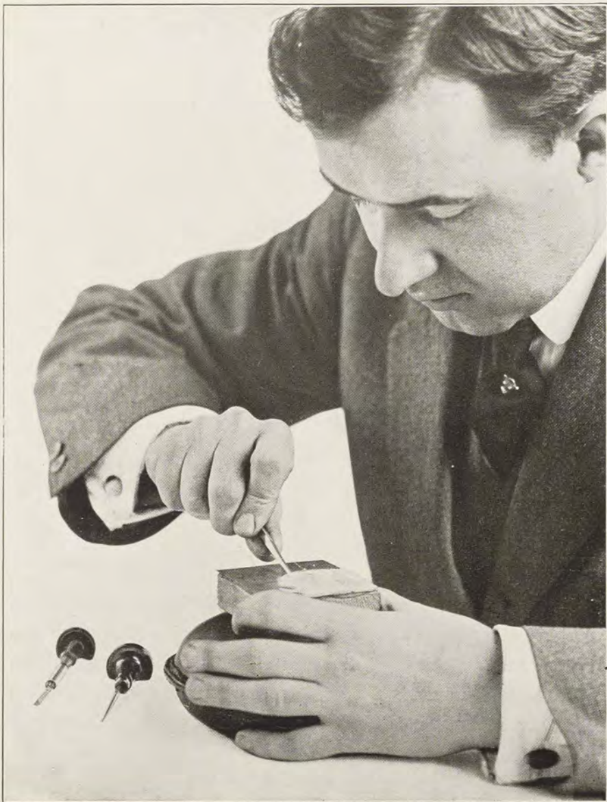
FIG. ONE Coarse Wriggling, Angle 20 Degrees, 36-37-38 flat, for Block and Old English Letters.
