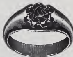
Oval Belcher ring as received with claws badly worn. Stone cannot be reset, as it would be too low to look well and the point would come below the inner circle of ring.
