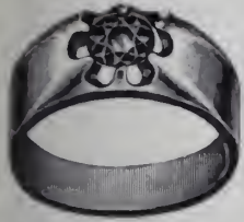
Flat Belcher ring as received with claws badly worn.
