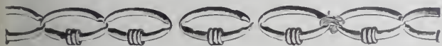
This cut shows part of a plain link chain as received for renewing
