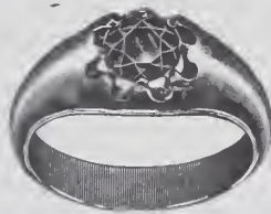
Oval Belcher ring as received with claws badly worn. Stone cannot be reset, as it would be too low to look well and the point would come below the inner circle of ring. (See cut No. 2 of flat Belcher.)
