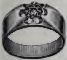
Flat Belcher ring as received with stone badly worn.
