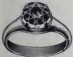
Tiffany ring as received with worn claws. Stone cannot be reset, as it would be too low to look well and the point would come below the inner circle of ring. (See cut No. 2 of flat belcher.)
