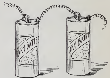
DRY BATTERIES, CONNECTED.
