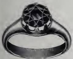
Tiffany ring as received with worn off claws. Stone cannot be reset, as it would be too low to look well and the point would come below the inner circle of ring.
