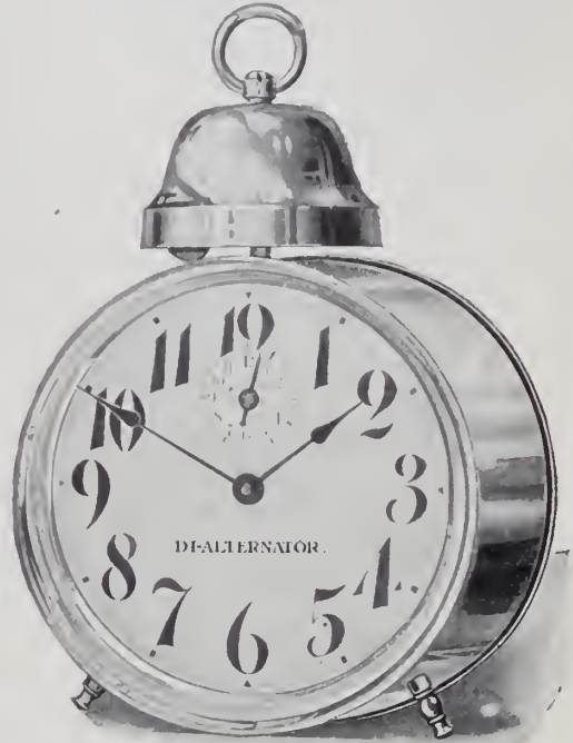
DI-ALTERNATOR. —30-hour time, Repeating Alarm, rings alternately every fifteen seconds for twelve minutes, with "shut-off" switch; extra large bell. Height, 7 in.; Dial, 4 1-2 in.; Case, seamless brass nickeled.
