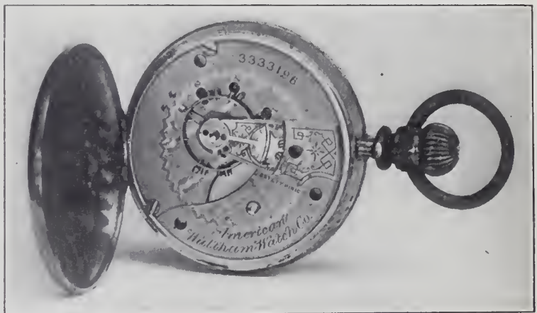
MOVEMENT STILL IN GOOD CONDITION AFTER 16 YEARS' INHUMATION.
