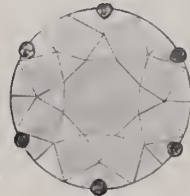
Effect of Yellow Gold Tips breaking into Surface of Diamond and decreasing its Beauty and Effectiveness.
