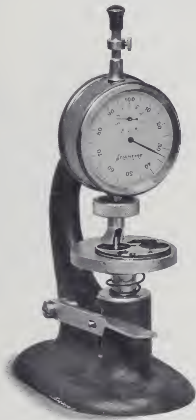
INSTRUMENT DESIGNED TO MEASURE DEPTH OF RECESS IN WATCH PLATES, ETC.
