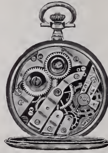
1389 Open face bridge model nickel silvered 7 jewel lever escapement quick train, pendant set, guaranteed mechanically perfect and accurate timekeeper, constructed on the interchangeable plan, bright silver nickel plates and bridges. Concave display winding wheels.
