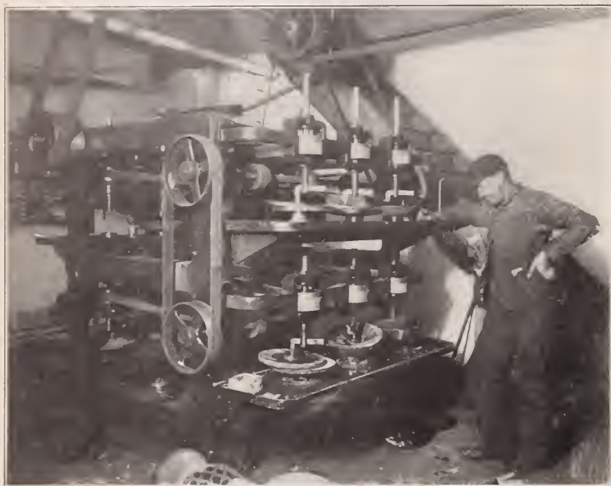
MODERN LENS GRINDER CARRYING 12 DISKS, 18 INCHES IN DIAMETER.
