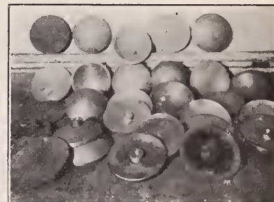
LARGE SHELLS FOR GRINDING SPHERICAL OR SPHERO-CYLINDRICAL LENSES.
