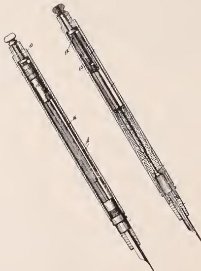
In a fountain-pen, a barrel having a valve-seat, a plunger held to travel in the barrel, a valve controlled by the plunger, adapted for engagement with the said seat, and means for operating the plunger.
