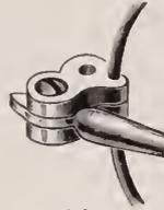
Can remove temple without disturbing lens.
