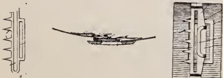
A belt buckle provided with a buckle-frame, a hook on the back of the frame, a toothed bar on the back of the said frame and spaced therefrom, and a plate extending from the said bar and spaced from the frame
