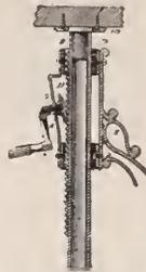
In an adjustable support for optical instruments, a metallic stand of tripod or like form comprising upwardly-converging legs, a guide-forming collar between the upper ends of such legs, headed screws inserted from within outwardly to fixedly unite said legs and collar, and a bushing of Babbitt metal or the like within said collar which fastens said screws and forms a central guide-bore.
