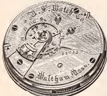
No. 53. Nickel Movement, 15 Jewels in Gold settings, Safety Pinion, Hardened and Tempered Breguet Hair-Spring, Compensation Balance, Patent Regulator, Double Sunk Dial.
