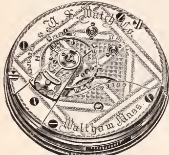
No. 40. Fine Nickel Movement, 17 Ruby Jewels in Gold settings, Safety Pinion, Hardened and Tempered Breguet Hair-Spring, Compensation Balance, Adjusted to heat, cold and positions, Patent Regulator, Double Sunk Dial.
