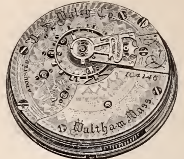
No. 79. First Quality Nickel Movement, 17 Ruby Jewels in Gold Settings, Safety Pinion, Hardened and Tempered Breguet Hair-Spring, Compensation Balance, Adjusted to Heat, Cold, Positions and Isochronism, Patent Regulator, Double Sunk Dial. This movement is specially adapted for Railway Service.
