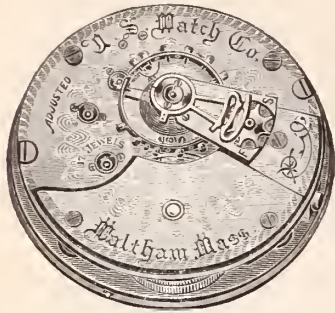
No. 80. Fine Nickel Movement, 17 Ruby Jewels in Gold settings, Safety Pinion, Hardened and Tempered Breguet Hair-Spring, Compensation Balance, Adjusted to heat, cold and positions; Patent Regulator, Double Sunk Dial.
