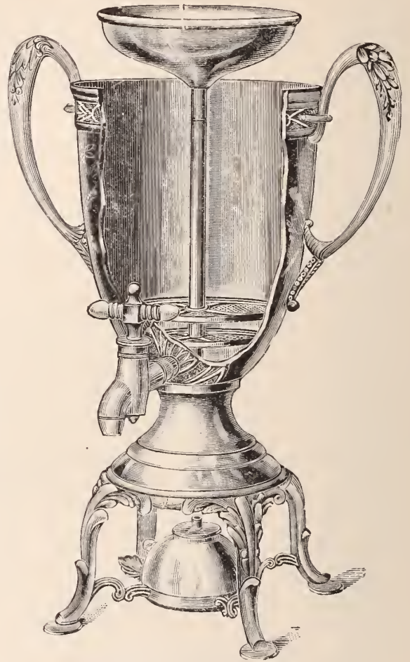
COFFEE PERCOLATOR. Cut showing inside Filtering, Etc.
