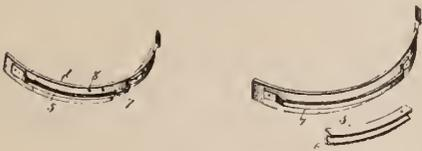
or slidable holder having a groove running from end to end and a series of screw-holes, the retaining screws by which the holder is fastened to the case, the spring upon which the holder rests, and the securing-strip resting in said groove in the holder and having its ends secured to the spring.
