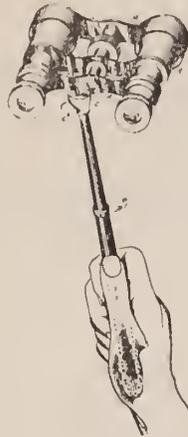
tion that is adapted to engage with and be thereby secured to a handle, cane, or other equivalent support, of a bow or shackle jointed to said socket, whereby to turn upon an axis longitudinally thereof, and means for locking such bow or shackle in one of its extremes of movement.
