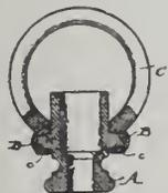
bow having its ends provided with journal-holes, swiveled upon said arms or ears, with a taper formed between the adjacent surfaces of the ends of the bow about the journal-holes and the arms or ears of the pendant, the arms or ears projecting through the journal-holes on the ends of the bow.
