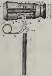
handle for said glass, provided with a segment gear which is pivoted to said handle and fitted to mesh into the gearing of said movable tubes, said segment gear having a lever fitted to be operated by a finger of the hand of the user.
