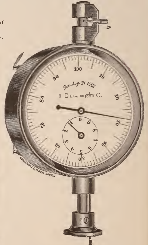
JAW AND DEPTH GAUGE. Patented Aug. 21, 1883. .001 of a centimeter or .001 of an inch, $14.00. .01 of a centimeter or .01 of an inch, $8.00.
