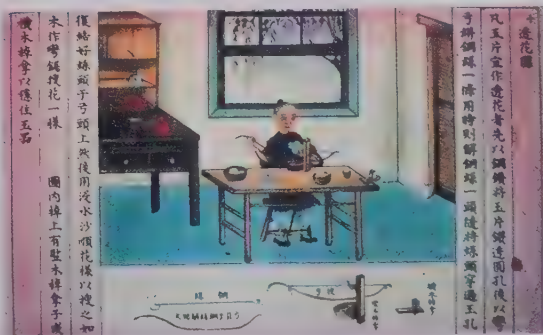
6. OPEN WORK If a piece is to be carved in openwork, it must first be pierced along the lines of the design by a narrow drill called a diamond borer, and then worked
