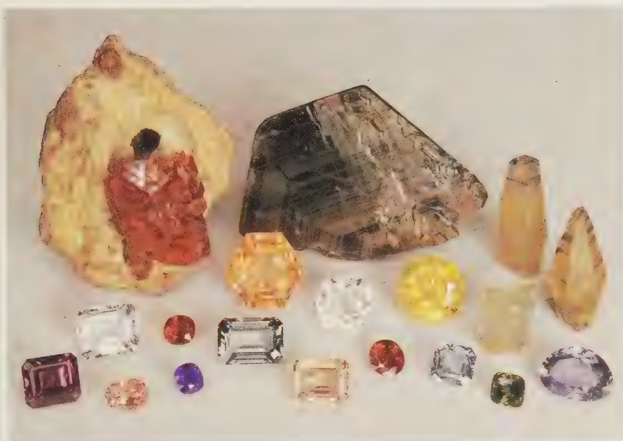
1 Corundum – Ruby crystal in matrix (top left), rough sapphire (top centre), three corundum crystals (right), and cut stones
