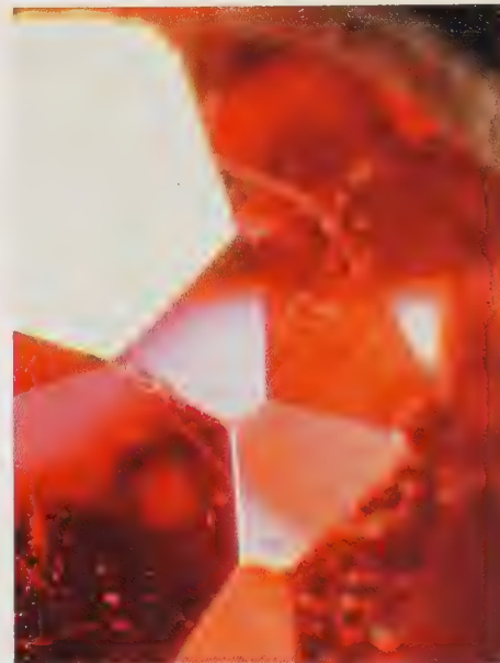
117 The junction (curved line) in a doublet
