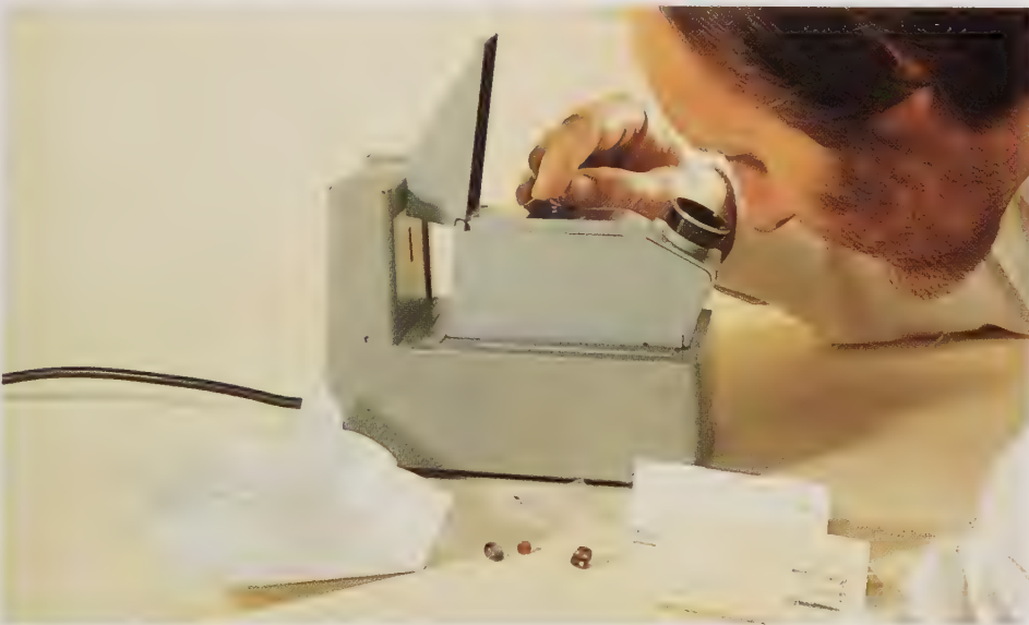
139 Refractometer in use, and views down the eye-piece
