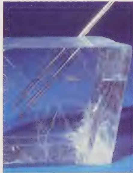
19 Double refraction in calcite
