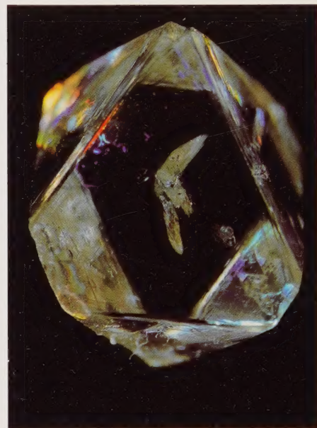
15 Cleavages in a diamond crystal
