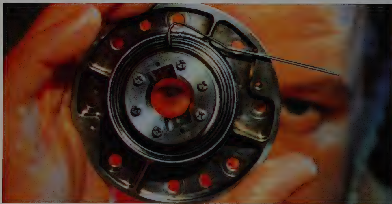
The diamond window (centre) of the Pioneer space probe sent to Venus
