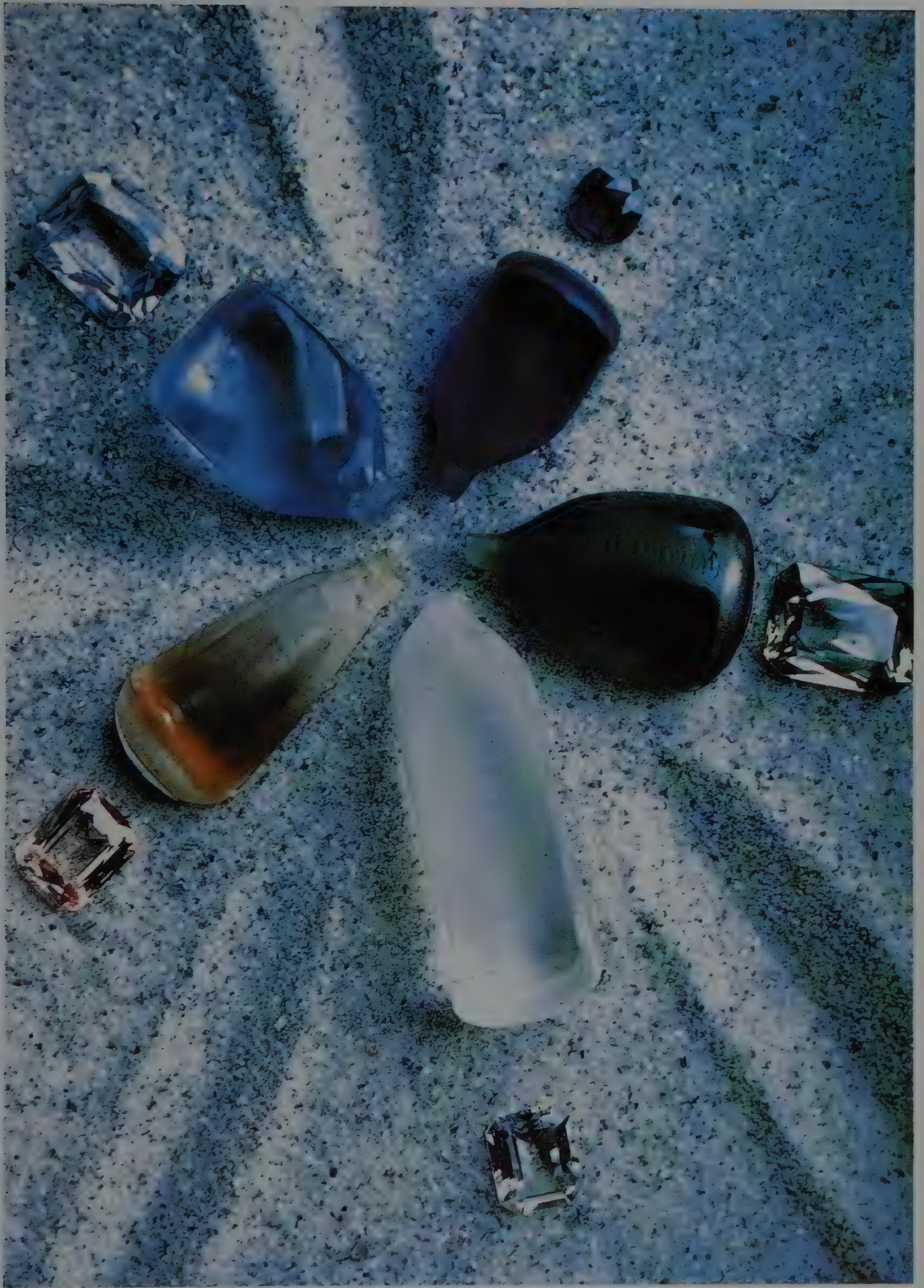
A selection of artificial gems – showing the crystal rod shapes from which they were cut.
