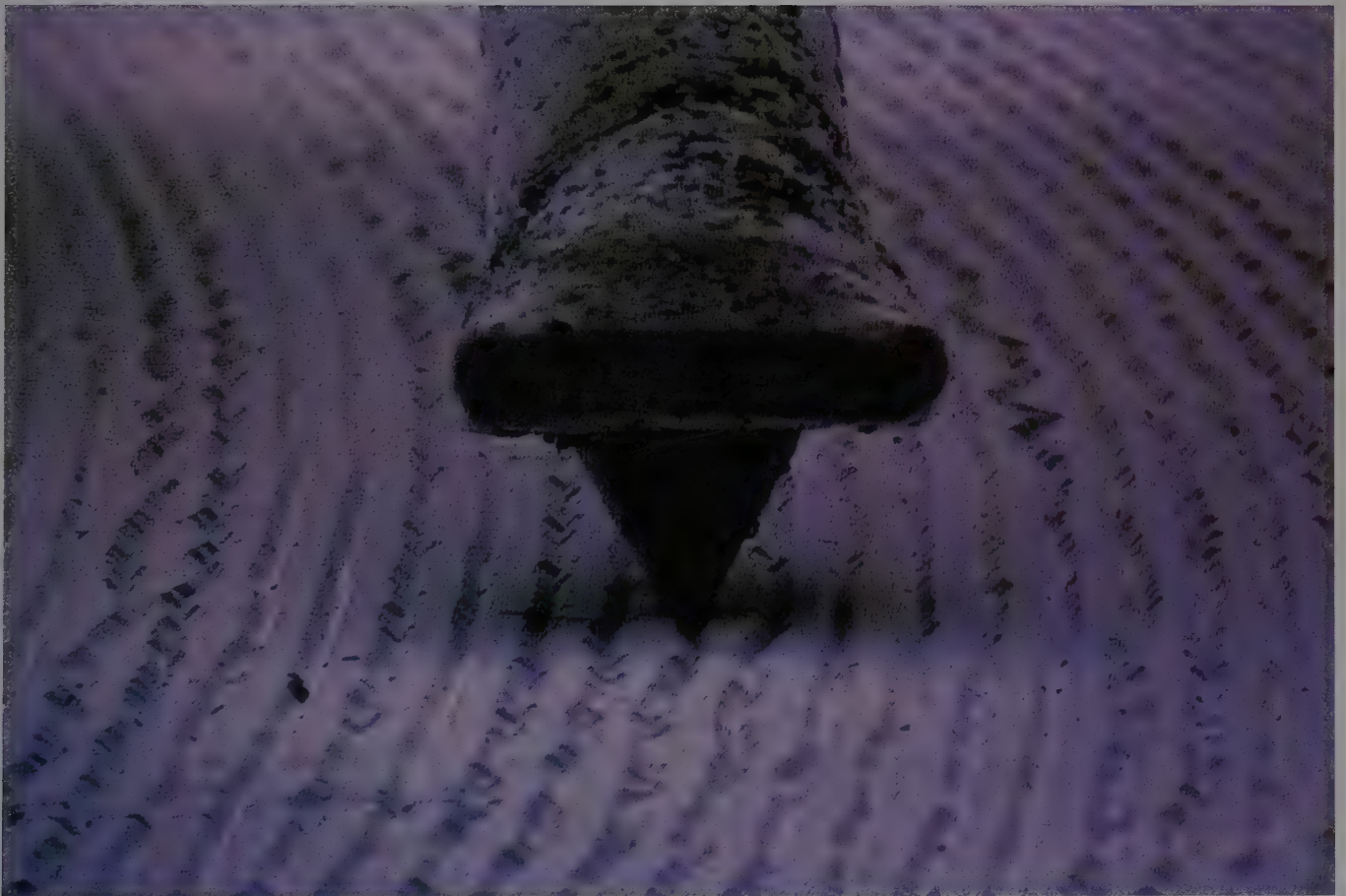
An electron microscope photograph of a diamond stylus in a vinyl record groove
