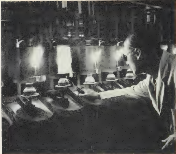
1. A bank of Verneuil chalumeaux in operation (Reproduced by courtesy of Salford Electrical Instruments Ltd.)
