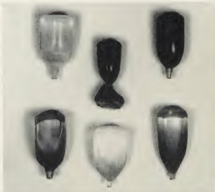
2. Boules of synthetic corundum (upper row) and spinel (lower row) (Photo by B. W. Anderson)
