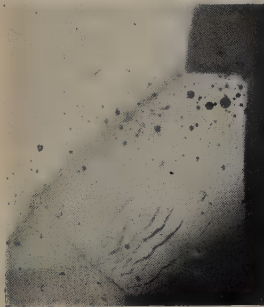
4. BUBBLES AND CRACK- LIKE MARKINGS
