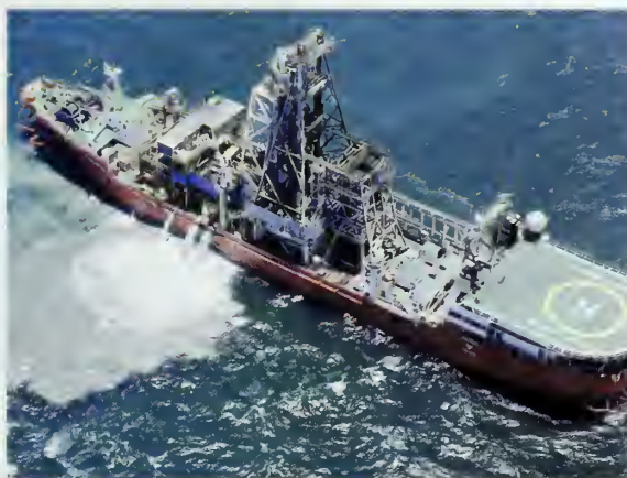
▲ Marine diamonds are retrieved from the sea using ships that vacuum the sand off the seabeds.
