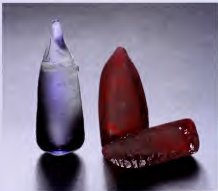
● Boules of synthetic ruby and synthetic sapphire
