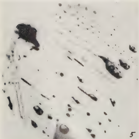
Fig. 12-5. TOPAZ. 75X. Drop-shaped, liquid-filled cavities with bubbles of gas. Called two-phase inclusions. Found in other species.
