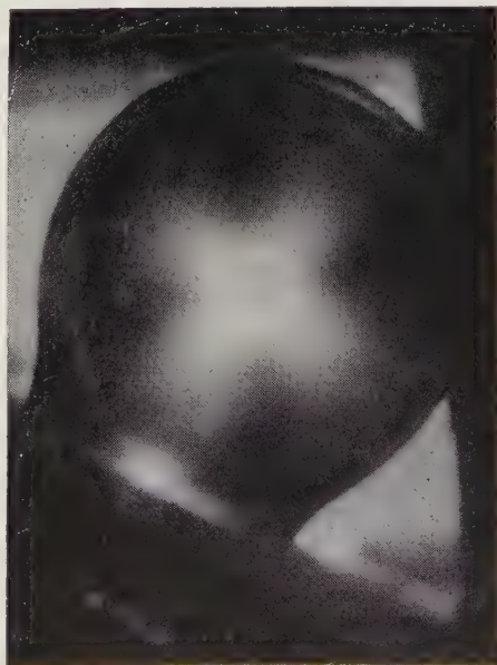
Fig. 17-13. Circularly polarized uniaxial optic figure as usually seen in quartz.
