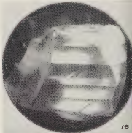
Fig. 12-16. FELDSPAR. 10X. Twinning observed in polarized light. Common to several species of feldspar. Not visible in nonpolarized light. Does not un-
