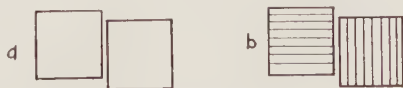
Fig. 20-2. (a) The windows of the dichroscope are usually seen offset like this. (b) The direction of vibration of light rays as seen through the dichroscope.
