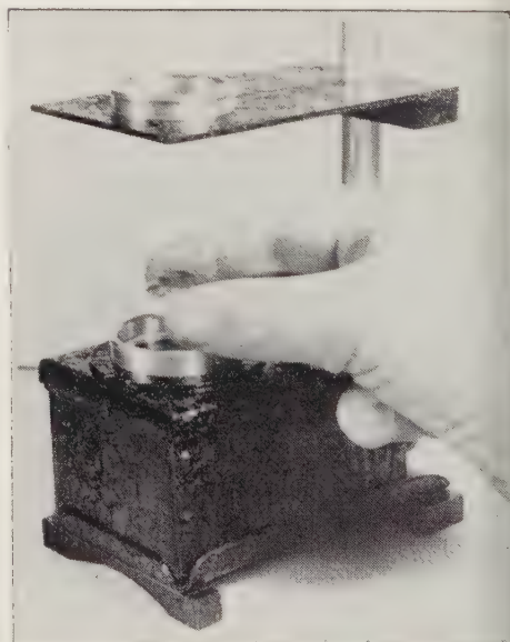
Fig. 17-4. How a stone is held by hand in the polariscope.
