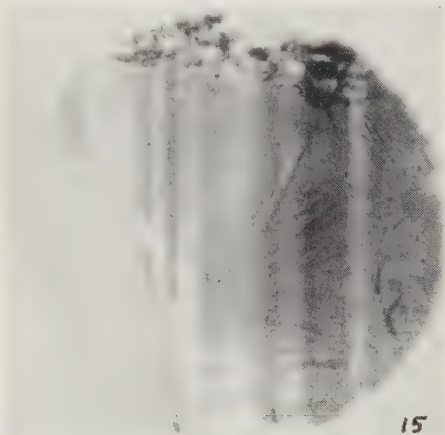
Fig. 12-15. SAPPHIRE. 10X. Color zoning in blue sapphire from Ceylon.
