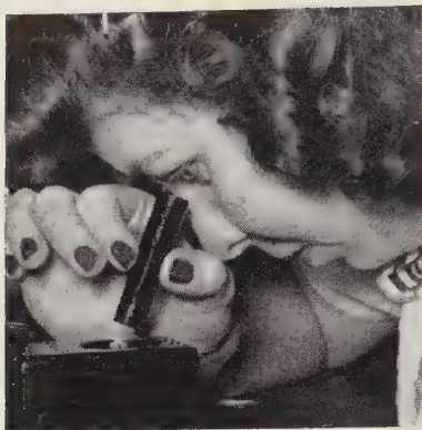
Fig. 20-3. The best way to use a dichroscope is to hold it close to the gem, using a good lamp such as this microscope substage lamp for illumination.
