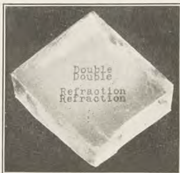
FIG. 73.—Calcite: variety, Iceland spar, showing double refraction. Big Timber, Montana.
