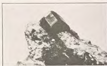
FIG. 174.—Crystal of garnet showing a combination of rhombic dodecahedron (large) and tetragonal trisoctahedron.
