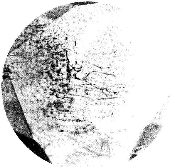
• Genuinelike gas inclusions in a synthetic ruby. 40x
