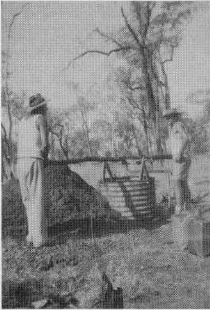
• Washing sapphire dirt in a 100 gallon tank of water with a spring sieve.
