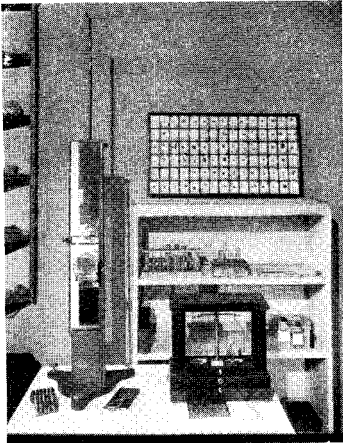
PHOTOGRAPH BY HERBERT LYMAN EMERSON, JR. The Jolly Balance and Diamond Balance for Specific Gravity Determinations. Dense Liquids and Acids for Metal Testing.
