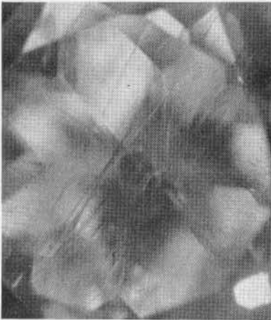
Fig. 2. Pronounced streaked effect in synthetic rutile (under 30x in dark-field illumination).
